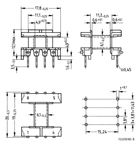
Hole arrangement View in mounting direction
