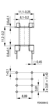
Hole arrangement View in mounting direction
