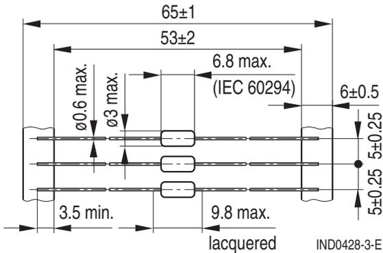
Minimum lead spacing 10 mm
