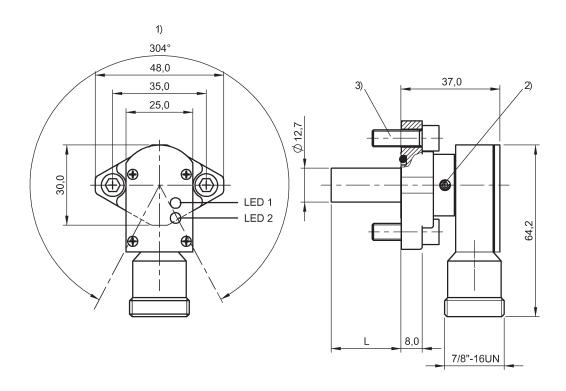
1) Housing rotatable by  $304^{\circ}$  2) Tightening torque 1...1.5 Nm 3) Tightening torque 16.5 Nm
