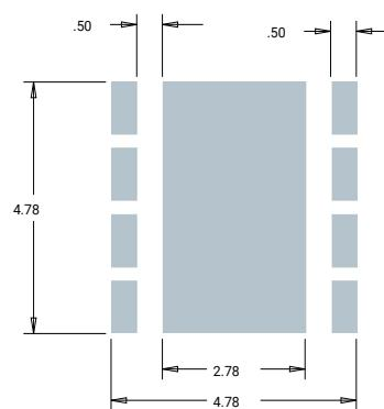
**Recommended PCB Solder Pad**
