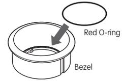
2. Remove bezel and red o-ring from housing. There are two o-rings in this assembly: one is red, one is orange.
