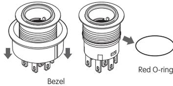
6. Align tab inside of the bezel with keyway on housing and bring bezel back into its original position.
