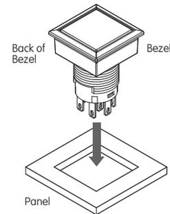
8. Attach mounting nut behind panel and tighten. Make sure that bezel and actuator fit properly and that there is no space between bezel and panel. Do not overtighten.
