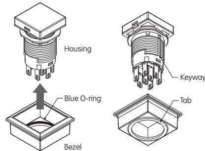
7. Before installing into panel, make sure that the square gasket is present at the back of the bezel. Align keyway on bezel with tab in panel and push switch all the way into the panel.
