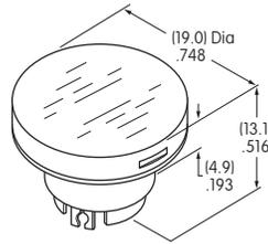
Material for Lens & Diffuser: Polycarbonate
