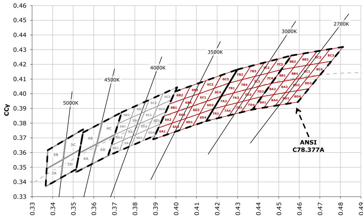
The following tables of order codes list flux minimums and chromaticity regions for the various categories of XLamp XP LEDs. For other flux and chromaticity combinations, contact Cree or an authorized distributor.
