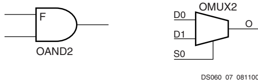
Figure 7: AND and MUX Symbols in Spartan-XL IOB
