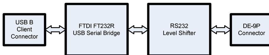
**Figure 1.2 USB2-F-1001 Block Diagram**
