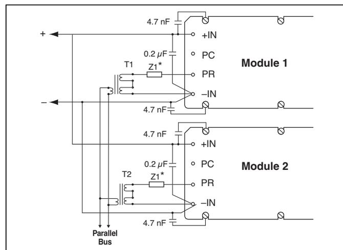
Figure 10 — Transformer-coupled interface.
