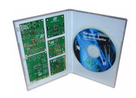
■ The **SO14\_TRIPLE** board supports a triple high-speed op-amp in the SO14 package with video application considerations.
