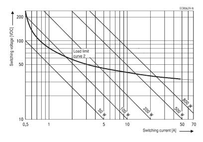
Load limit curve  $2 \stackrel{\triangle}{=} safe$  shutdown, no stationary arc (make contact)
