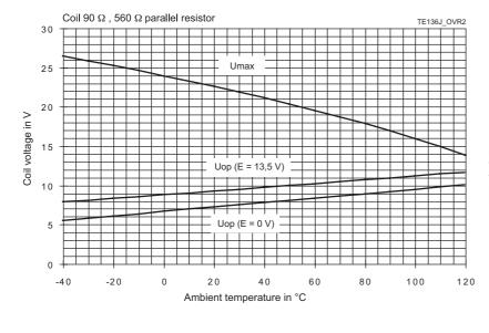
Does not take into account the temperature rise due to the contact current E = pre-energization Uop = operate voltage
