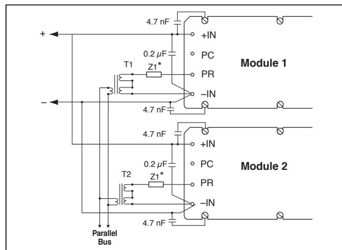
Figure 10 — Transformer-coupled interface.
