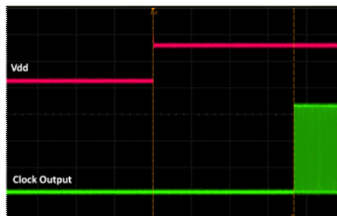
Figure 17. Startup Waveform vs. Vdd
