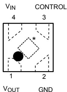
\*Center electrode should be connected to GND or Open
