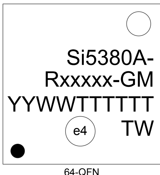
Figure 12.1. Si5380 Top Marking
