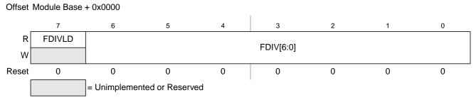
Figure 18-5. Flash Clock Divider Register (FCLKDIV)
