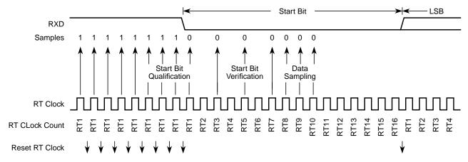
Figure 14-21. Receiver Data Sampling
