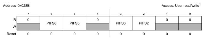
Figure 2-73. Port S Interrupt Flag Register (PIFS)
