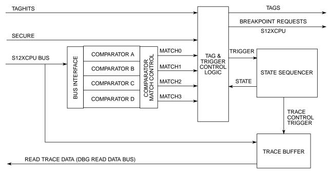
Figure 6-1. Debug Module Block Diagram
