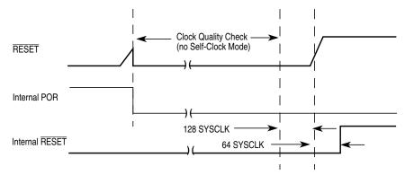
Figure 7-22. RESET Pin Tied to V<sub>DD</sub> (by a Pull-up Resistor)
