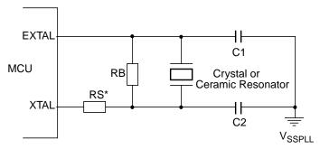
$<sup>^{\</sup>star}$  R  $_{\rm S}$  can be zero (shorted) when use with higher frequency crystals. Refer to manufacturer's data.
