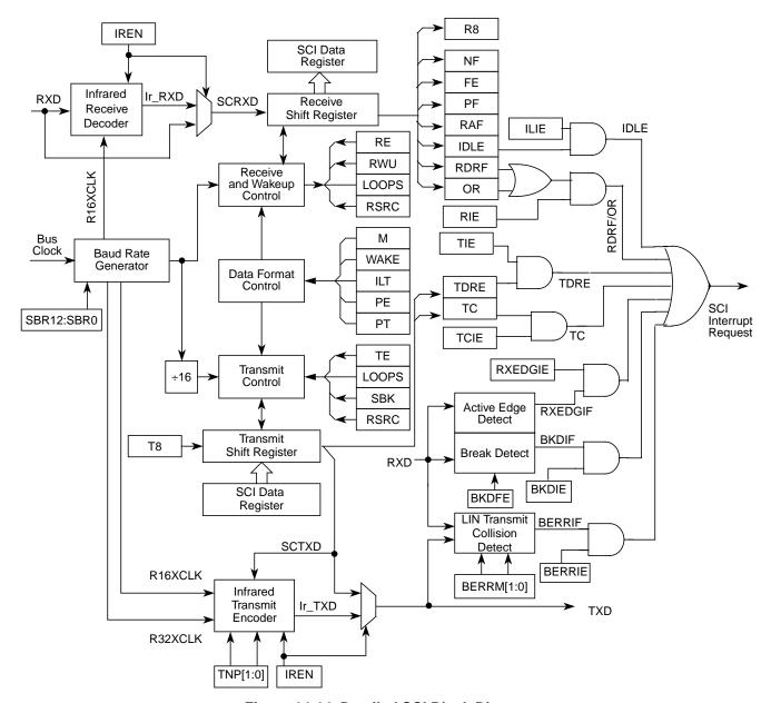
Figure 14-14. Detailed SCI Block Diagram
