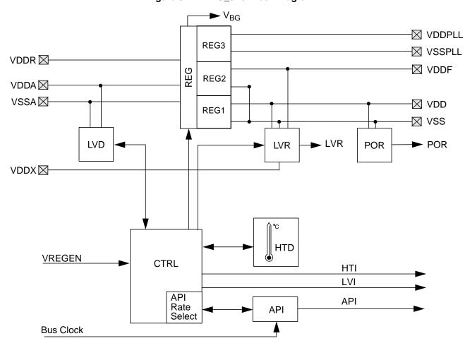
Figure 9-1. VREG\_3V3 Block Diagram
