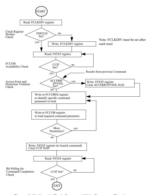
Figure 19-26. Generic Flash Command Write Sequence Flowchart
