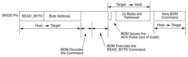
Figure 5-12. Handshake Protocol at Command Level
