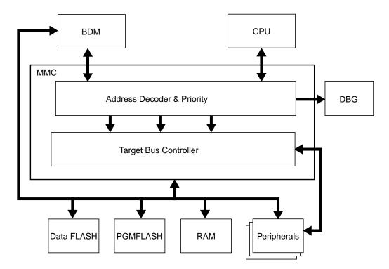
Figure 3-1. MMC Block Diagram
