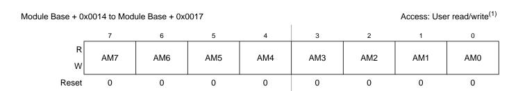
Figure 11-22. MSCAN Identifier Mask Registers (First Bank) — CANIDMR0-CANIDMR3
