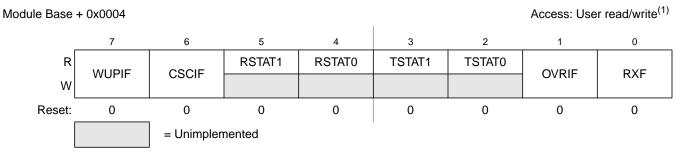
Figure 11-8. MSCAN Receiver Flag Register (CANRFLG)
