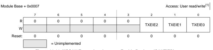
Figure 11-11. MSCAN Transmitter Interrupt Enable Register (CANTIER)
