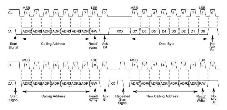
Figure 12-10. IIC-Bus Transmission Signals
