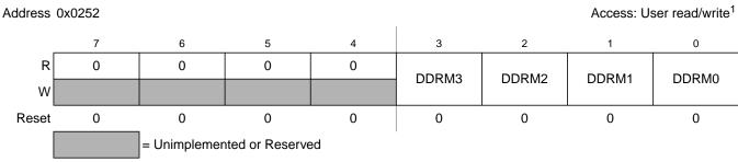
Figure 2-30. Port M Data Direction Register (DDRM)
