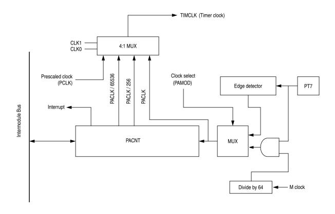
Figure 16-2. 16-Bit Pulse Accumulator Block Diagram
