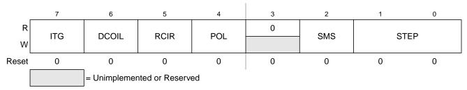
Figure 21-2. Return-to-Zero Control Register (RTZCTL)
