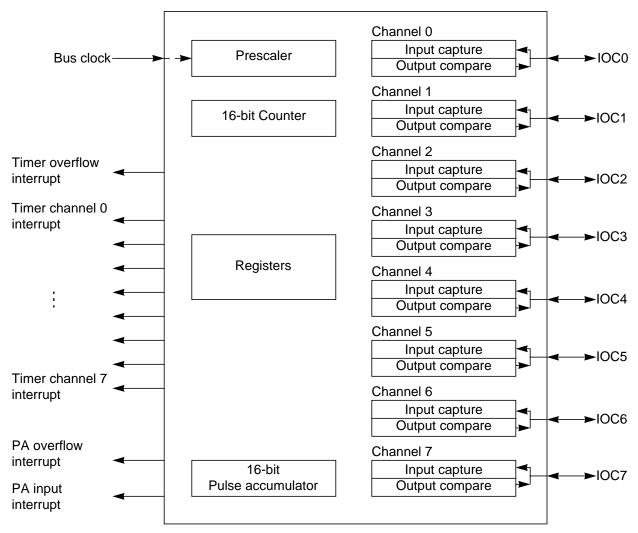
Figure 16-1. TIM16B8CV2 Block Diagram
