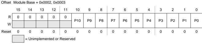
Figure 20-5. Motor Controller Period Register (MCPER) with DITH = 0
