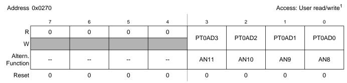
Figure 2-53. Port AD Data Register (PT0AD)
