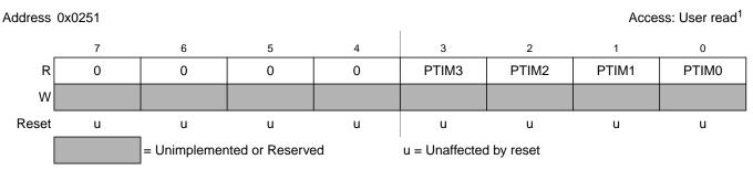
Figure 2-29. Port M Input Register (PTIM)
