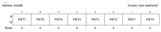
Figure 2-70. Port TInterrupt Enable Register (PIET)
