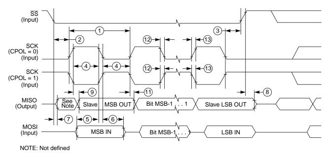
Figure A-12. SPI Slave Timing (CPHA = 1)
