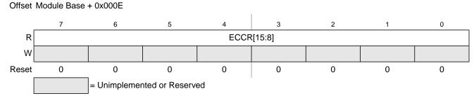
Figure 19-20. Flash ECC Error Results High Register (FECCRHI)
