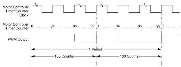
Figure 20-20. PWM Output: DITH = 1, MCAM[1:0] = 10, MCDC = 31, MCPER = 200, RECIRC = 0
