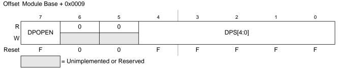
Figure 19-15. D-Flash Protection Register (DFPROT)
