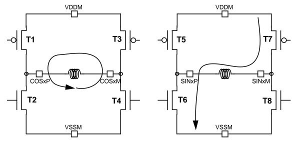
Figure 21-14. Current flow when STEP = 3, DCOIL = 1, ITG = 1
