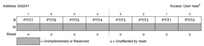
Figure 2-13. Port T Input Register (PTIT)
