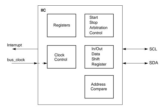
Figure 12-1. IIC Block Diagram
