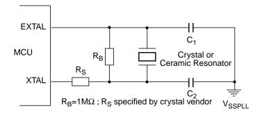
Figure 1-7. Full Swing Pierce Oscillator Connections (XCLKS = 1)
