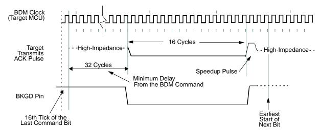
Figure 5-11. Target Acknowledge Pulse (ACK)
