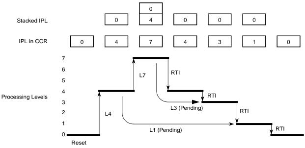
Figure 4-14. Interrupt Processing Example
