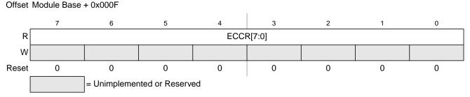
Figure 18-21. Flash ECC Error Results Low Register (FECCRLO)
