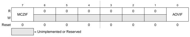
Figure 21-5. Stepper Stall Detector Flag Register (SSDFLG)
