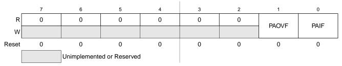
Figure 16-25. Pulse Accumulator Flag Register (PAFLG)
