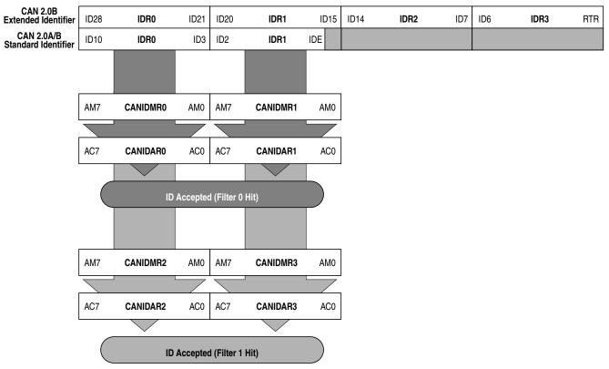
Figure 11-41. 16-bit Maskable Identifier Acceptance Filters
