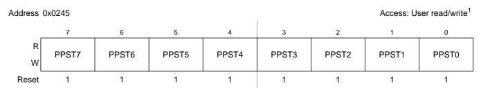
Figure 2-17. Port T Polarity Select Register (PPST)
