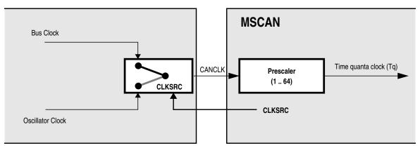
Figure 11-43. MSCAN Clocking Scheme
