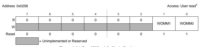
Figure 2-34. Port MWired-Or Mode Register
