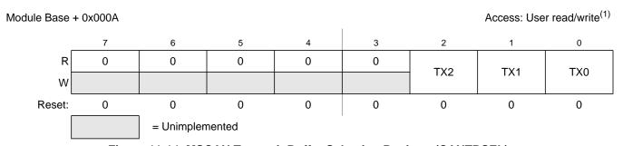
Figure 11-14. MSCAN Transmit Buffer Selection Register (CANTBSEL)
