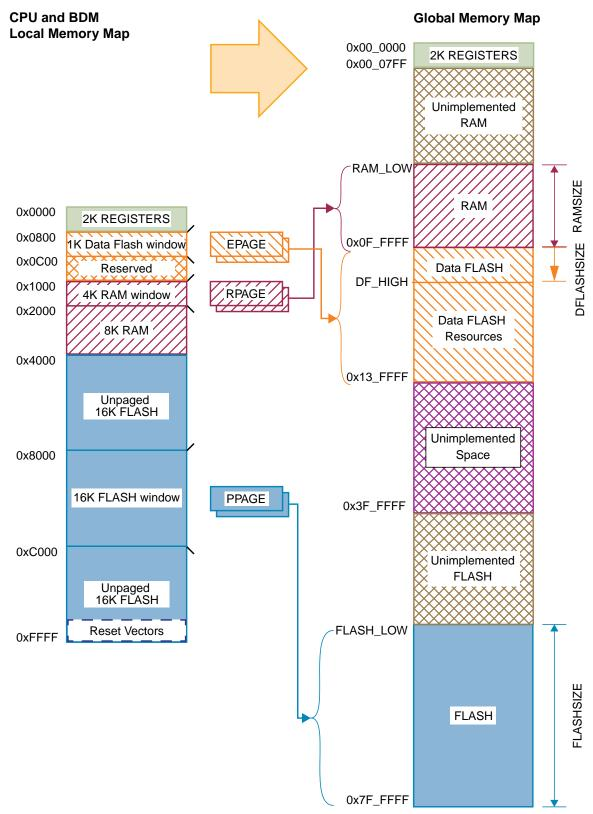
Figure 3-19. S12X CPU & BDM Global Address Mapping
