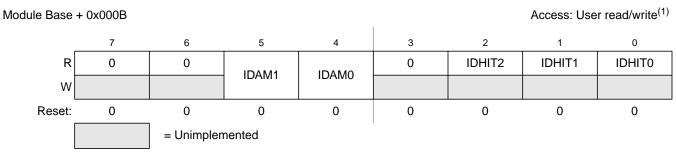
Figure 11-15. MSCAN Identifier Acceptance Control Register (CANIDAC)
