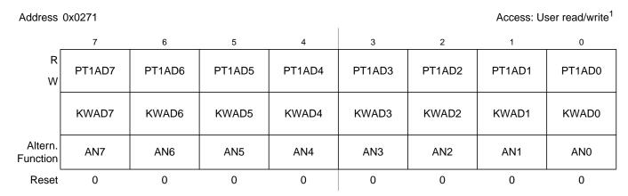
Figure 2-54. Port AD Data Register (PT1AD)
