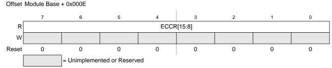
Figure 18-20. Flash ECC Error Results High Register (FECCRHI)
