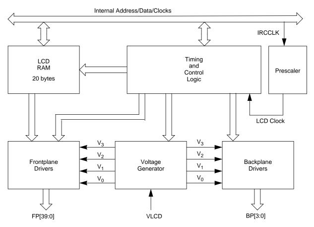
Figure 17-1. LCD40F4BV2 Block Diagram
