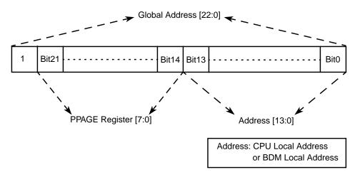
Figure 3-12. PPAGE Address Mapping
