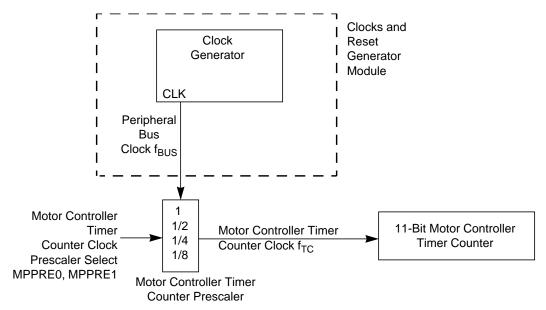
Figure 20-22. Motor Controller Counter Clock Selection
