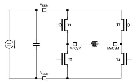
Figure 20-16. Output Transistor Assignment
