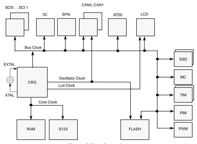
Figure 1-5. Clock Connections
