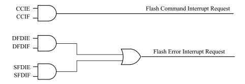
Figure 18-27. Flash Module Interrupts Implementation
