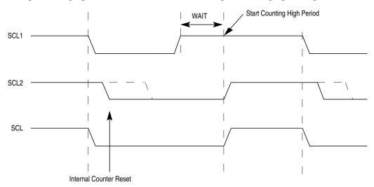
Figure 12-12. IIC-Bus Clock Synchronization
