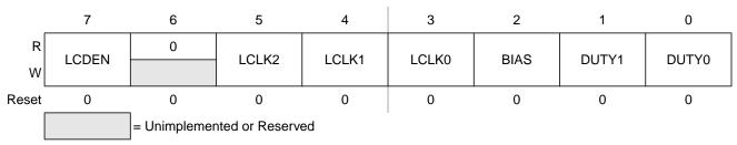
Figure 17-2. LCD Control Register 0 (LCDCR0)
