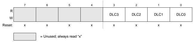
Figure 11-35. Data Length Register (DLR) — Extended Identifier Mapping
