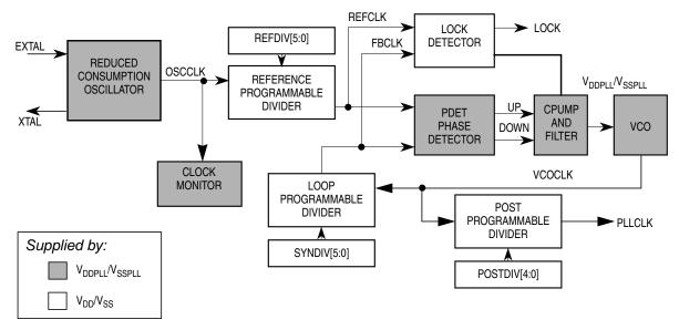
Figure 7-15. IPLL Functional Diagram
