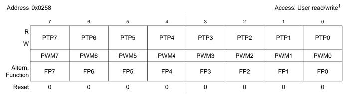
Figure 2-36. Port P Data Register (PTP)
