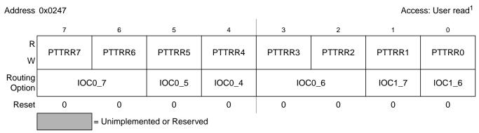
Figure 2-19. Port T Routing Register (PTTRR)
