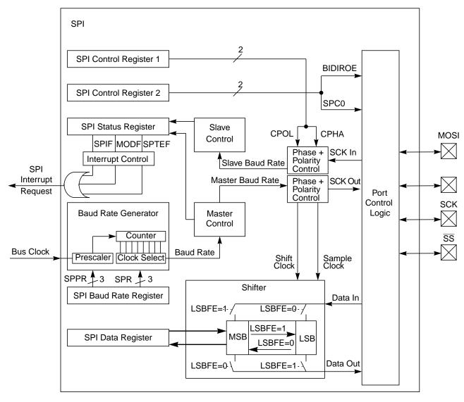
Figure 15-1. SPI Block Diagram
