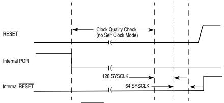
Figure 7-23. RESET Pin Held Low Externally
