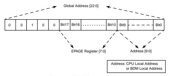
Figure 3-16. EPAGE Address Mapping
