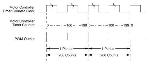
Figure 20-17. PWM Output: DITH = 0, MCAM[1:0] = 01, MCDC = 100, MCPER = 200, RECIRC = 0
