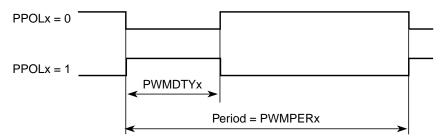
Figure 13-20. PWM Left Aligned Output Waveform
