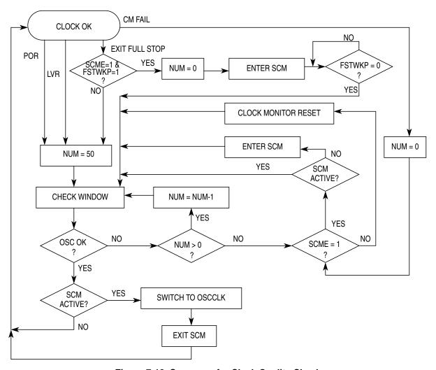
Figure 7-18. Sequence for Clock Quality Check
