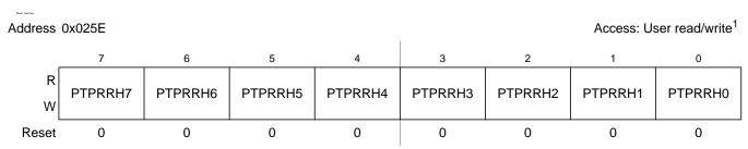
Figure 2-42. Port P Routing Register High (PTPRRH)
