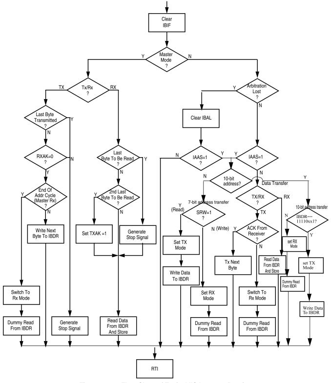
Figure 12-16. Flow-Chart of Typical IIC Interrupt Routine
