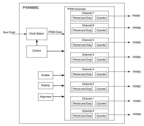
Figure 13-1. PWM Block Diagram
