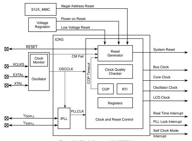
Figure 7-1. Block diagram of S12XECRG
