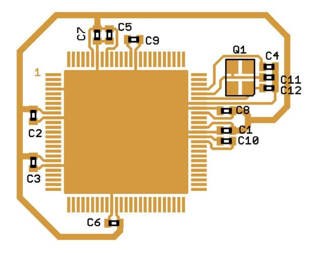
Figure C-2. 100-Pin QFP Recommended PCB Layout (Loop Controlled Pierce Oscillator)
