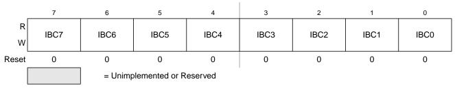
Figure 12-4. IIC Bus Frequency Divider Register (IBFD)
