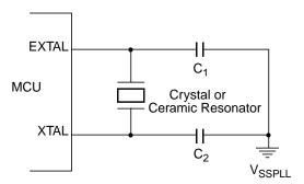
Figure 1-6. Loop Controlled Pierce Oscillator Connections (XCLKS = 0)
