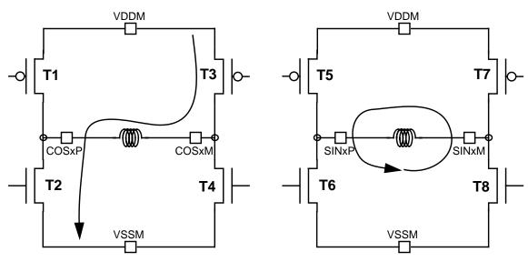
Figure 21-13. Current flow when STEP = 2, DCOIL = 1, ITG = 1
