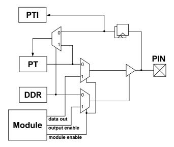
Figure 2-94. Illustration of I/O pin functionality
