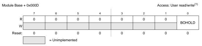
Figure 11-17. MSCAN Miscellaneous Register (CANMISC)
