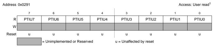
Figure 2-79. Port U Input Register (PTIU)
