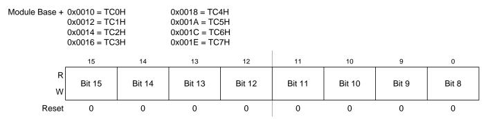
Figure 16-22. Timer Input Capture/Output Compare Register x High (TCxH)
