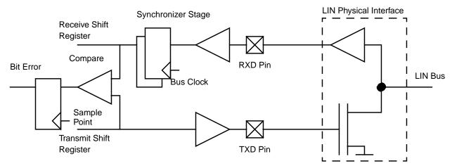
Figure 14-18. Collision Detect Principle
