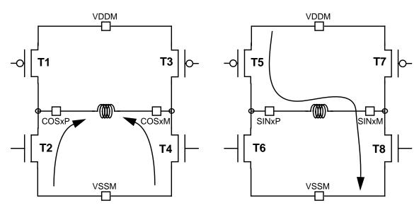
Figure 21-12. Current Flow when STEP = 1, DCOIL = 1, ITG = 0, RCIR = 1
