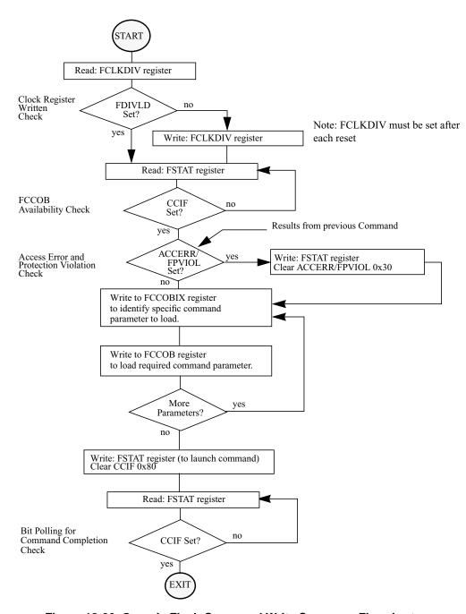
Figure 18-26. Generic Flash Command Write Sequence Flowchart
