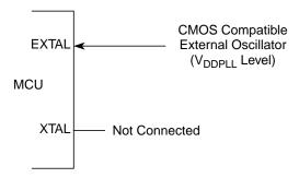
Figure 8-4. External Clock Connections (FSP mode selected)
