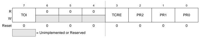
Figure 16-19. Timer System Control Register 2 (TSCR2)
