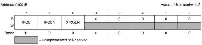
Figure 2-10. IRQ Control Register (IRQCR)
