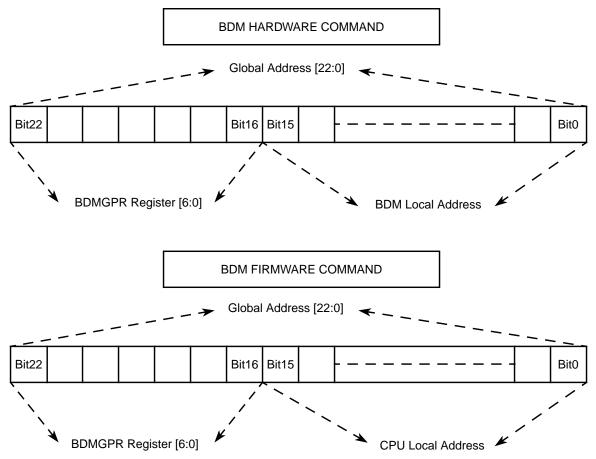
Figure 3-18. BDMGPR Address Mapping
