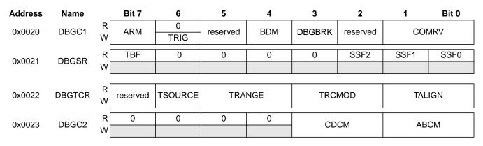
Figure 6-2. Quick Reference to S12XDBG Registers
