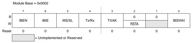
Figure 12-6. IIC Bus Control Register (IBCR)
