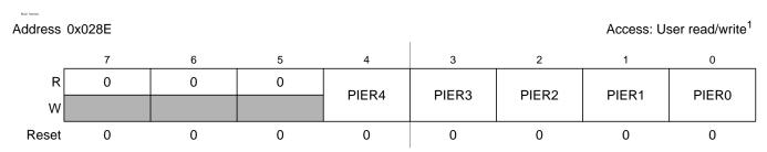
Figure 2-76. Port R Interrupt Enable Register (PIER)
