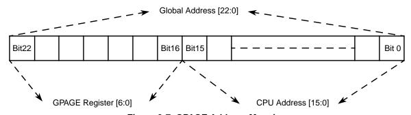
Figure 3-7. GPAGE Address Mapping
