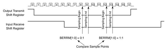
Figure 14-19. Timing Diagram Bit Error Detection
