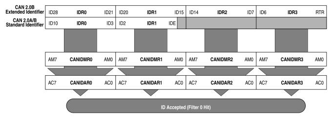
Figure 11-40. 32-bit Maskable Identifier Acceptance Filter
