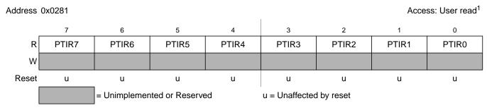
Figure 2-63. Port R Input Register (PTIR)
