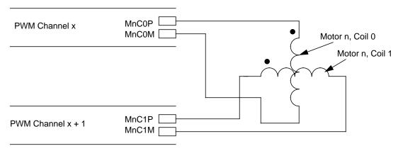
Figure 20-10. Typical Dual Full H-Bridge Mode Configuration
