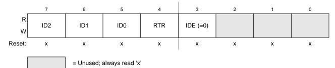
Figure 11-31. Identifier Register 1 — Standard Mapping
