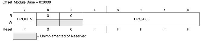
Figure 18-15. D-Flash Protection Register (DFPROT)
