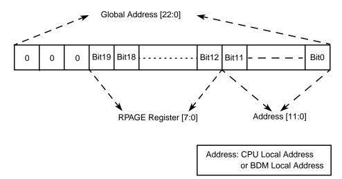
Figure 3-14. RPAGE Address Mapping
