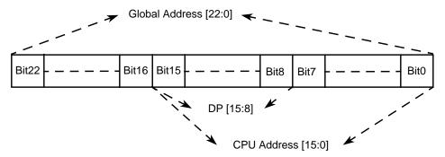
Figure 3-9. DIRECT Address Mapping
