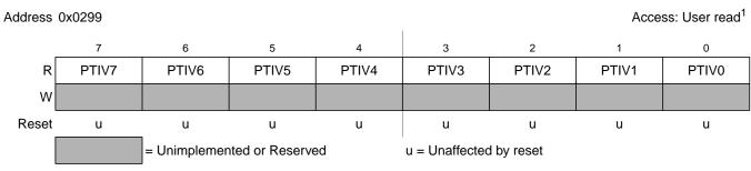
Figure 2-87. Port V Input Register (PTIV)
