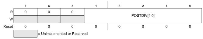
Figure 7-5. S12XECRG Post Divider Register (POSTDIV)
