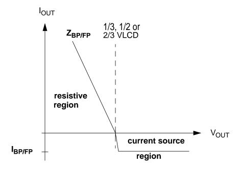
Figure A-8. buffer output characteristic
