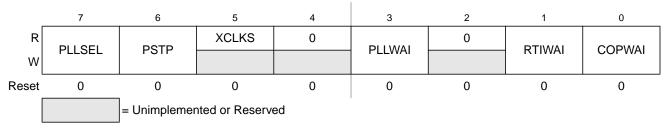
Figure 7-8. S12XECRG Clock Select Register (CLKSEL)
