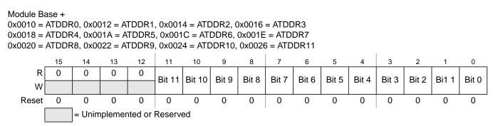
Figure 10-15. Right justified ATD conversion result register (ATDDR*n*)
