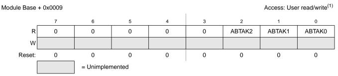
Figure 11-13. MSCAN Transmitter Message Abort Acknowledge Register (CANTAAK)
