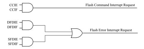
Figure 19-27. Flash Module Interrupts Implementation
