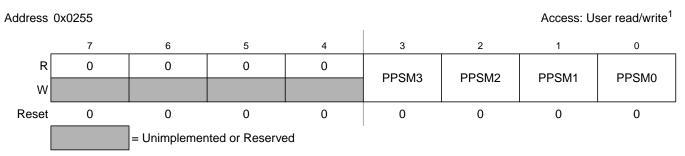
Figure 2-33. Port M Polarity Select Register (PPSM)
