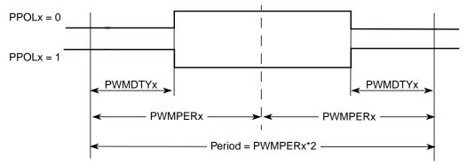
Figure 13-22. PWM Center Aligned Output Waveform
