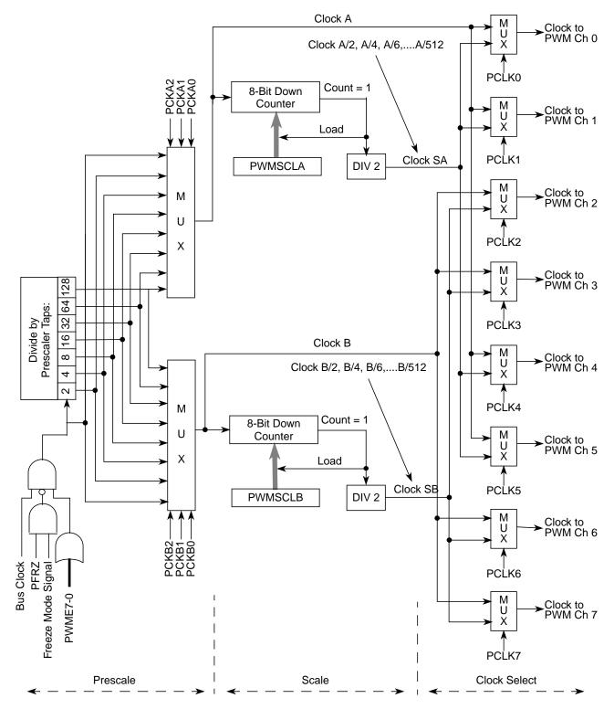
Figure 13-18. PWM Clock Select Block Diagram
