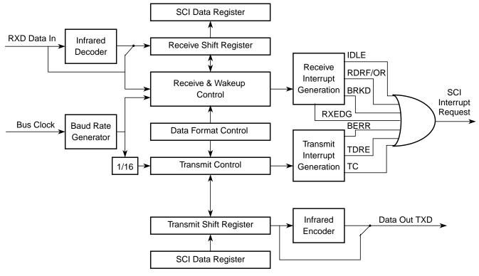
Figure 14-1. SCI Block Diagram
