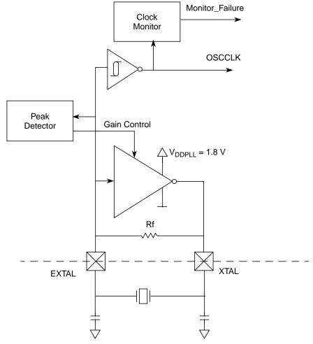
Figure 8-1. XOSC Block Diagram
