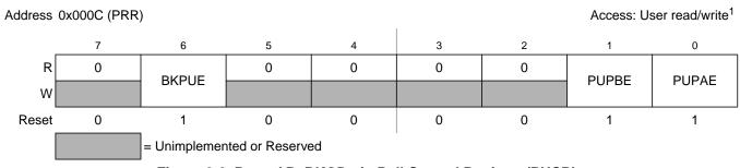
Figure 2-6. Ports AB, BKGD pin Pull Control Register (PUCR)
