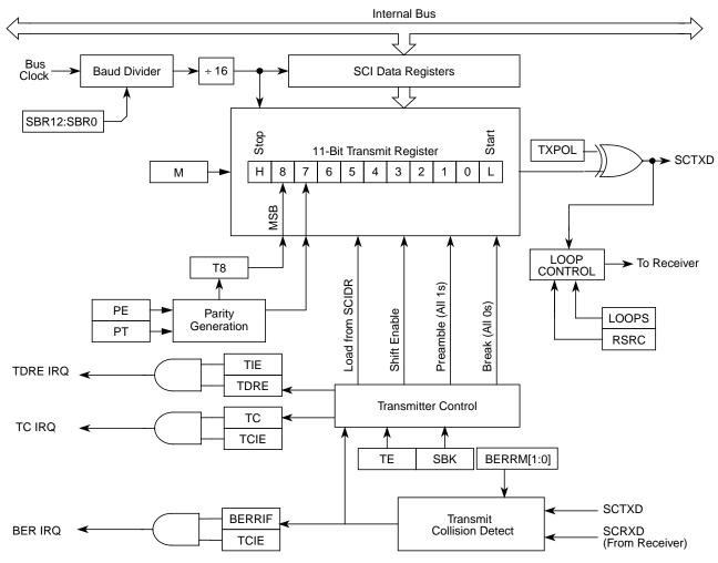
Figure 14-16. Transmitter Block Diagram
