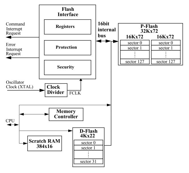
Figure 18-1. FTMR256K1 Block Diagram
