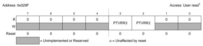
Figure 2-93. Port V Routing Register (PTVRR)
