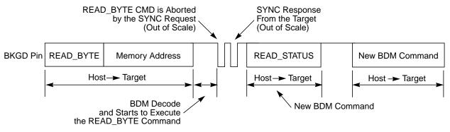
Figure 5-13. ACK Abort Procedure at the Command Level
