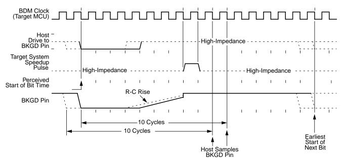
Figure 5-9. BDM Target-to-Host Serial Bit Timing (Logic 1)
