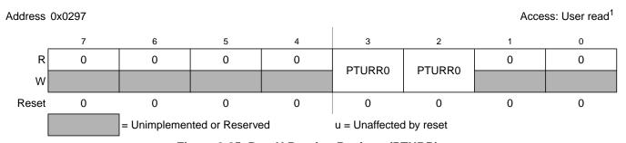
Figure 2-85. Port U Routing Register (PTURR)
