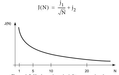
Figure A-5. Maximum bus clock jitter approximation
