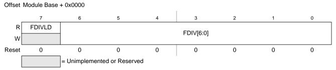
Figure 19-5. Flash Clock Divider Register (FCLKDIV)
