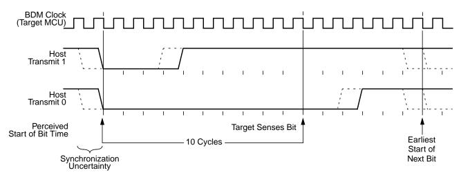
Figure 5-8. BDM Host-to-Target Serial Bit Timing
