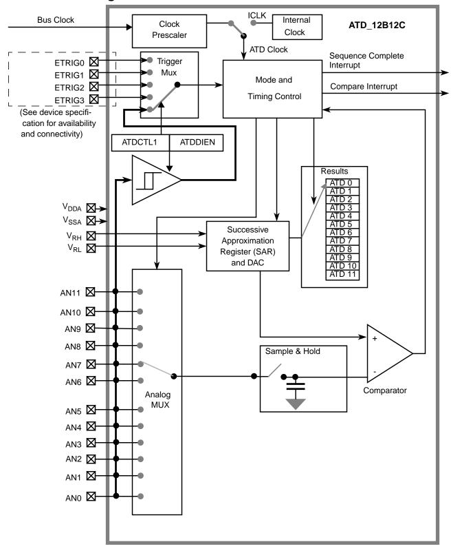
Figure 10-1. ADC12B12C Block Diagram
