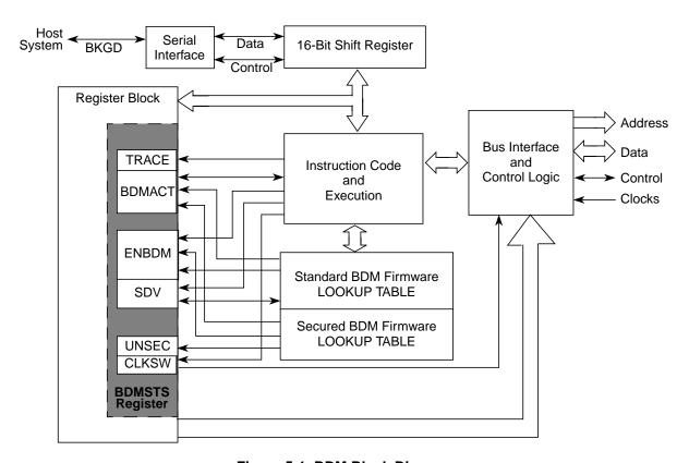
Figure 5-1. BDM Block Diagram
