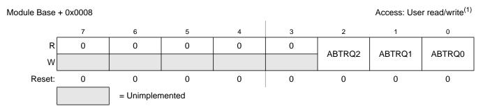
Figure 11-12. MSCAN Transmitter Message Abort Request Register (CANTARQ)
