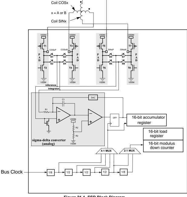
Figure 21-1. SSD Block Diagram
