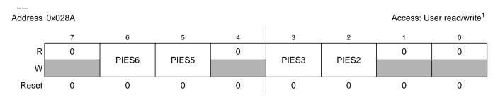
Figure 2-72. Port S Interrupt Enable Register (PIES)
