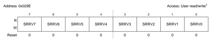
Figure 2-92. Port V Polarity Select Register (SRRV)
