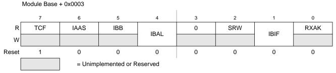
Figure 12-7. IIC Bus Status Register (IBSR)
