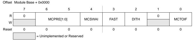
Figure 20-3. Motor Controller Control Register 0 (MCCTL0)
