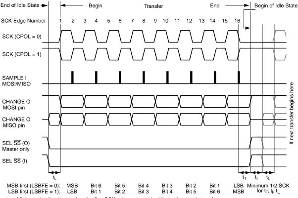
t<sub>1</sub> = Minimum leading time before the first SCK edge, not required for back-to-back transfers
