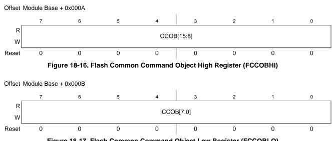
Figure 18-17. Flash Common Command Object Low Register (FCCOBLO)
