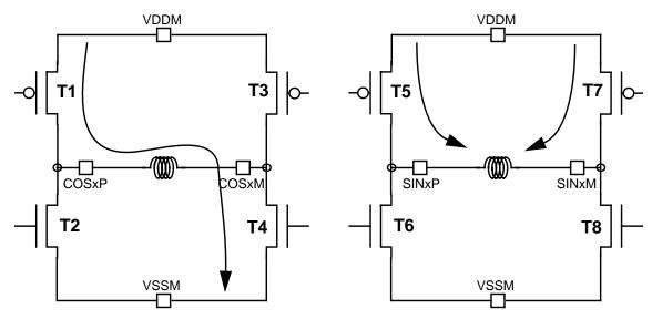
Figure 21-11. Current Flow when STEP = 0, DCOIL = 1, ITG = 0, RCIR = 0
