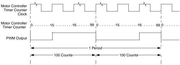
Figure 20-18. PWM Output: DITH = 1, MCAM[1:0] = 01, MCDC = 31, MCPER = 200, RECIRC = 0
