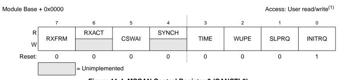
Figure 11-4. MSCAN Control Register 0 (CANCTL0)
