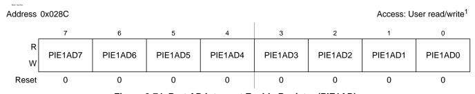
Figure 2-74. Port AD Interrupt Enable Register (PIE1AD)
