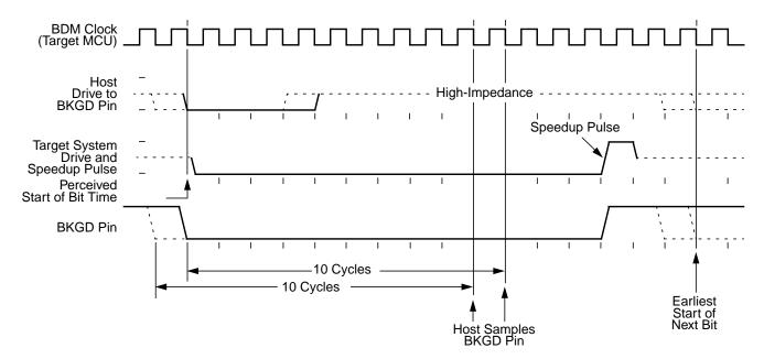
Figure 5-10. BDM Target-to-Host Serial Bit Timing (Logic 0)
