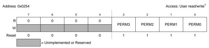
Figure 2-32. Port M Pull Device Enable Register (PERM)
