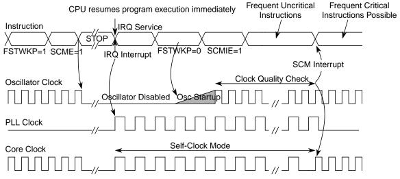
Figure 7-20. Fast Wake-up from Full Stop Mode: Example 2
