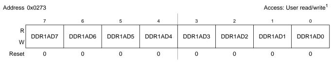
Figure 2-56. Port AD Data Direction Register (DDR1AD)
