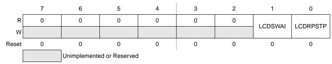
Figure 17-3. LCD Control Register 1 (LCDCR1)
