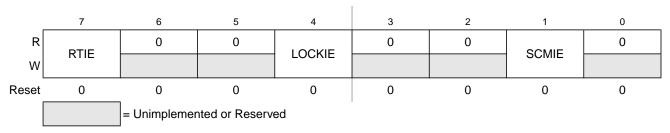
Figure 7-7. S12XECRG Interrupt Enable Register (CRGINT)
