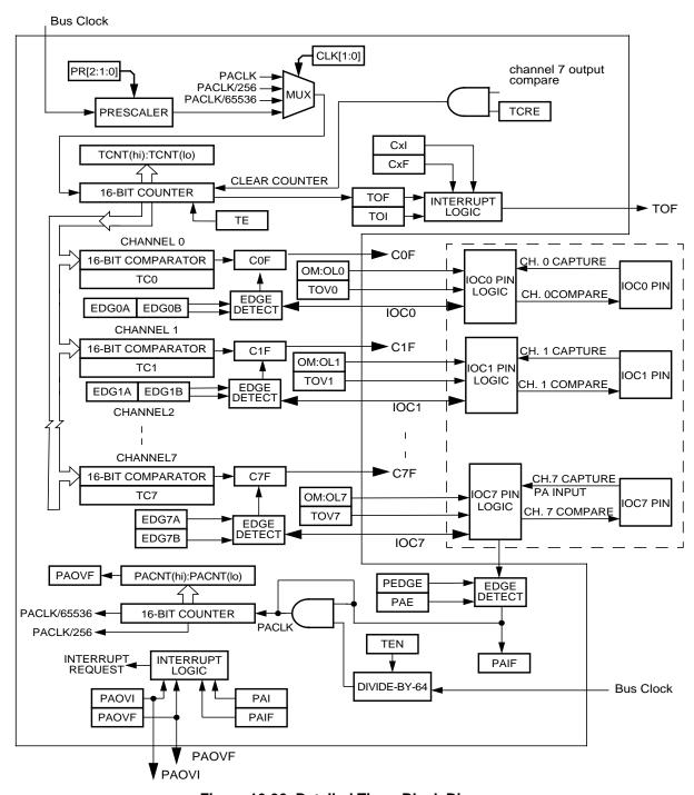
Figure 16-30. Detailed Timer Block Diagram
