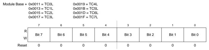
Figure 16-23. Timer Input Capture/Output Compare Register x Low (TCxL)
