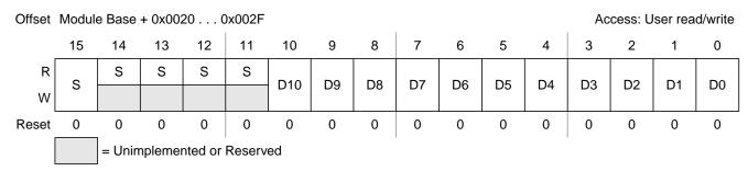
Figure 20-8. Motor Controller Duty Cycle Register x (MCDCx) with FAST = 0
