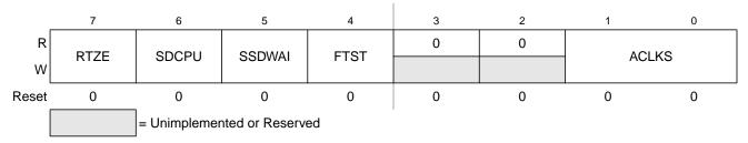
Figure 21-4. Stepper Stall Detector Control Register (SSDCTL)
