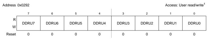
Figure 2-80. Port U Data Direction Register (DDRU)
