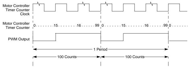
Figure 20-19. PWM Output: DITH = 1, MCAM[1:0] = 01, MCDC = 30, MCPER = 200, RECIRC = 0
