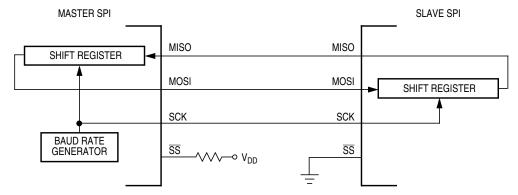
Figure 15-11. Master/Slave Transfer Block Diagram
