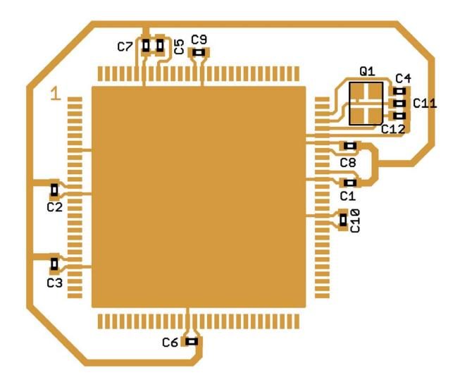
Figure C-1. 112-Pin LQFP Recommended PCB Layout (Loop Controlled Pierce Oscillator)
