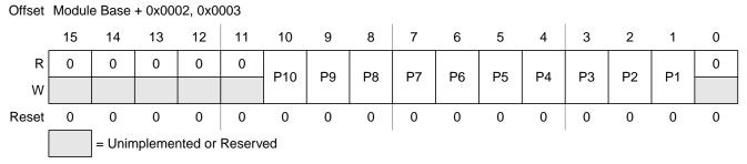
Figure 20-6. Motor Controller Period Register (MCPER) with DITH = 1
