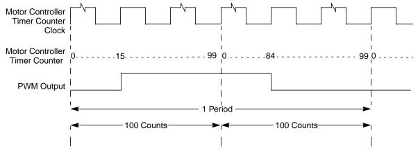
Figure 20-21. PWM Output: DITH = 1, MCAM[1:0] = 11, MCDC = 31, MCPER = 200, RECIRC = 0
