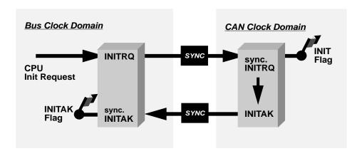
Figure 11-45. Initialization Request/Acknowledge Cycle
