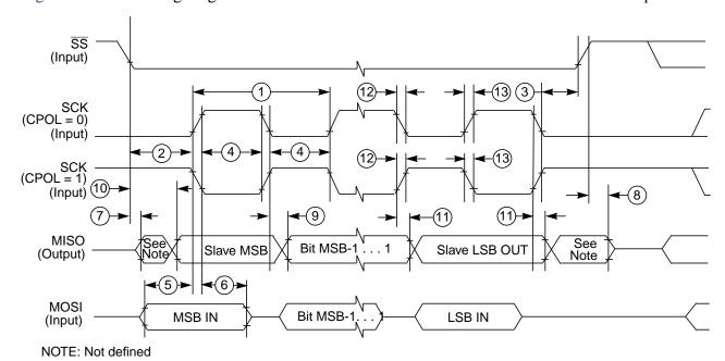
Figure A-11. SPI Slave Timing (CPHA = 0)
