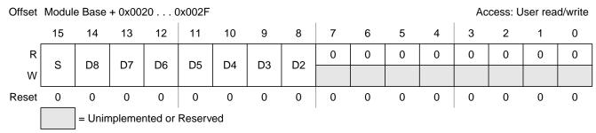
Figure 20-9. Motor Controller Duty Cycle Register x (MCDCx) with FAST = 1
