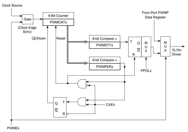
Figure 13-19. PWM Timer Channel Block Diagram
