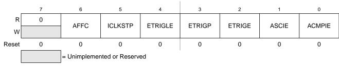
Figure 10-5. ATD Control Register 2 (ATDCTL2)
