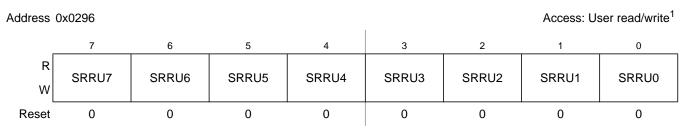
Figure 2-84. Port U Polarity Select Register (SRRU)
