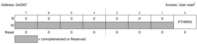
Figure 2-51. Port HRouting Register (PTHRR)
