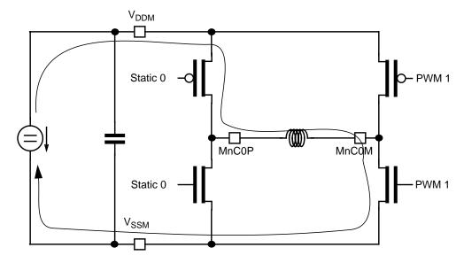
Figure 20-12. PWM Active Phase, RECIRC = 0, S = 0
