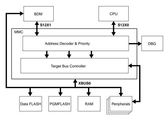
Figure 3-20. MMC Block Diagram
