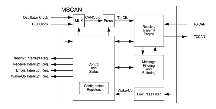
Figure 11-1. MSCAN Block Diagram
