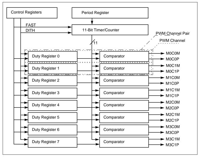
Figure 20-1. MC10B8C Block Diagram
