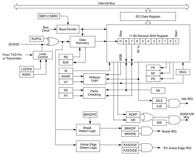
Figure 14-20. SCI Receiver Block Diagram
