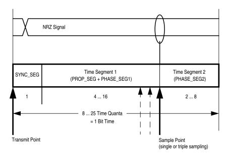
Figure 11-44. Segments within the Bit Time
