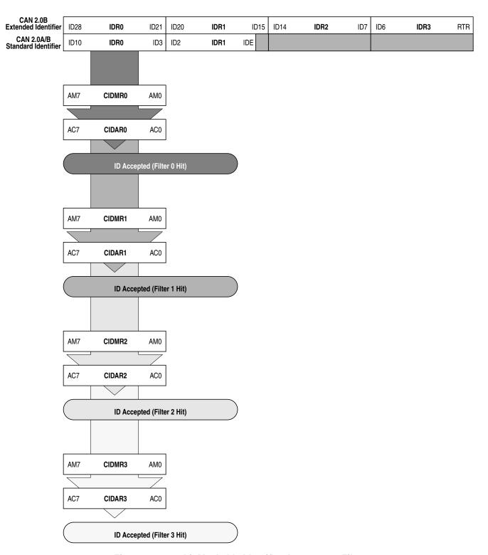
Figure 11-42. 8-bit Maskable Identifier Acceptance Filters
