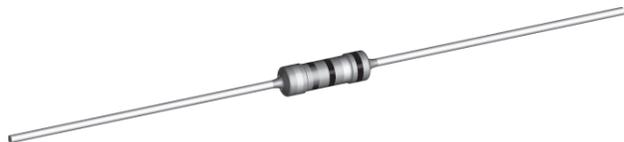
A homogeneous film of metal alloy is deposited on a high grade ceramic body. After a helical groove has been cut in the resistive layer, tinned connecting leads of electrolytic copper are welded to the end-caps.
