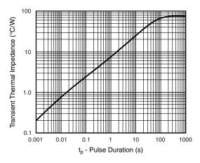
Fig. 5 - Typical Transient Thermal Impedance
