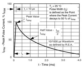
Fig. 3 - Pulse Waveform
