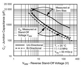
Fig. 4 - Typical Junction Capacitance Uni-Directional
