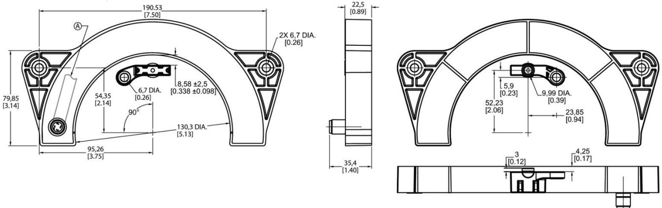
**A** = Cable direction for right angle connector
