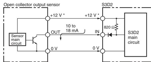
Note: Terminals (7) and (10), and (9) and (12) are connected internally.
