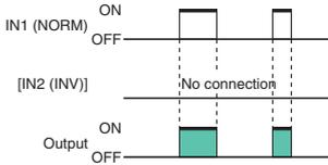
Note: When connecting only one Sensor, be sure to set the input selector switch for the unconnected Sensor to INV.
