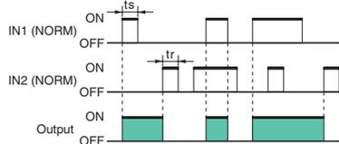
Note:  $t_s \geq 2ms$ ,  $t_r \geq 2ms$
