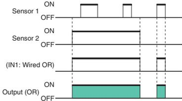
Note: When two Sensors are wired OR and then receive input (IN1 or IN2), OR operation is possible.
