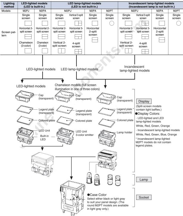
Note: The above diagram for LED lamp-lighted and incandescent lamp-lighted models shows the M2PJ model.
