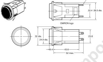
Note: Use a panel thickness of 0.5 mm for tab terminals #110 and solder terminals.
