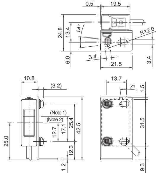
Note 1: Center of optical axis (through-beam type)
