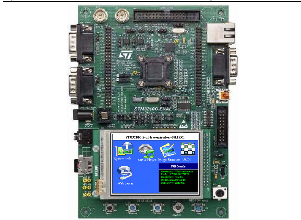
Figure 1. STM3210C-EVAL board with touch screen navigation
