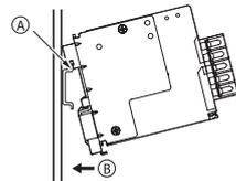
To remove the S8VM from the DIN Rail, insert a screwdriver into section C and pull the S8VM away from the Rail.
