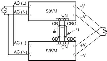
Use 2-conductor shielded cable as connection wire (\* 1).
