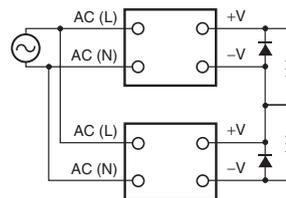
**Note: 1.** If the load is short-circuited, a reverse voltage may be applied inside the Power Supply unit, and this may possibly cause the deterioration or damage of the Power Supply unit. Connect the diode as shown in the figure. Use the following guidelines to select the diode to be connected.
