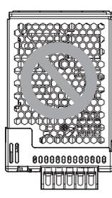
**Note:** 1. Improper mounting will interfere with heat dissipation and may occasionally result in deterioration or damage of internal parts.
