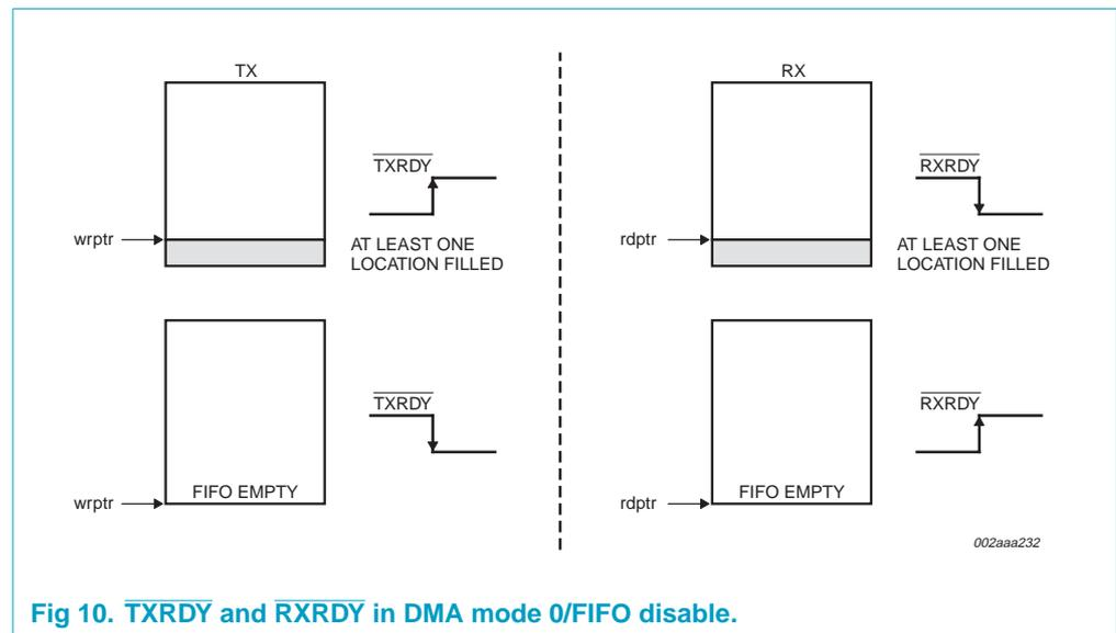
Fig 10.  $\overline{\text{TXRDY}}$  and  $\overline{\text{RXRDY}}$  in DMA mode 0/FIFO disable.
