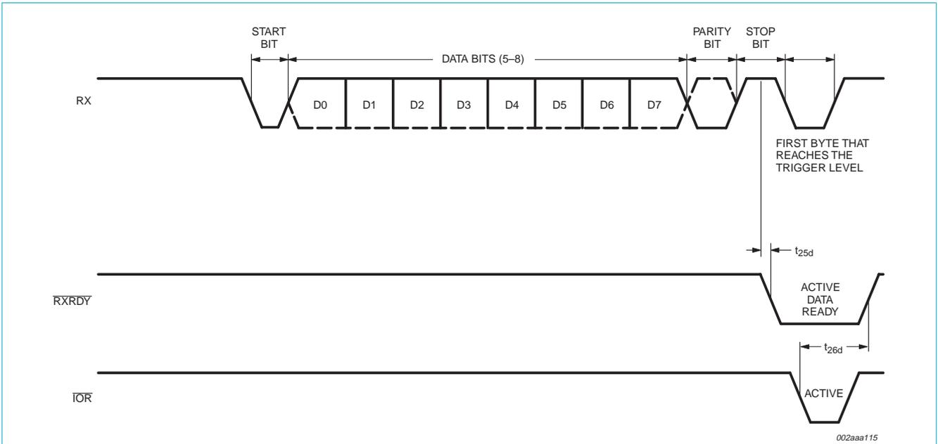
Fig 20. Receive ready timing in FIFO mode.
