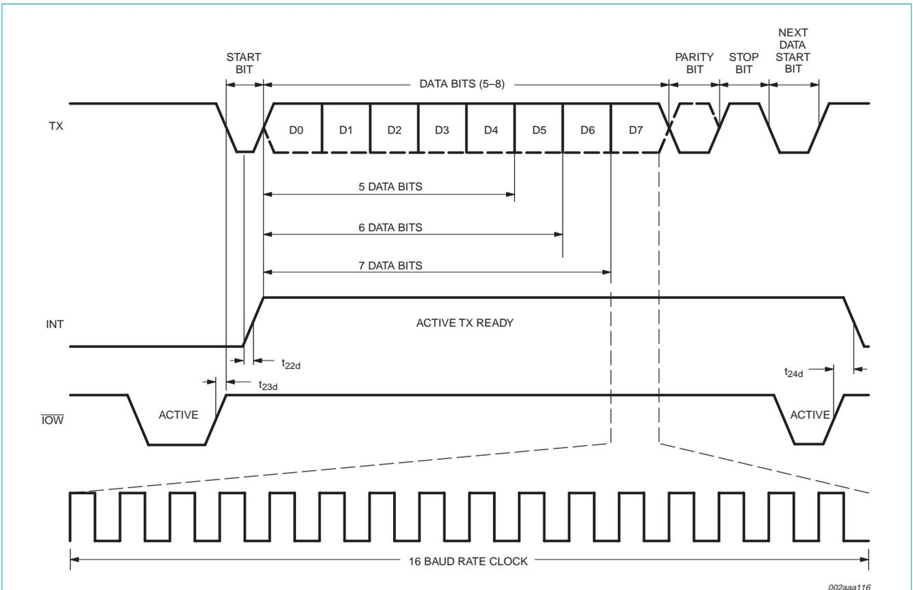
Fig 21. Transmit timing.
