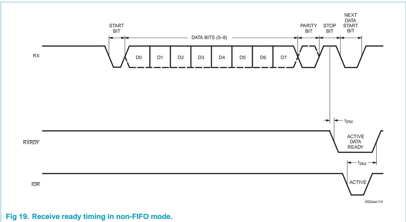
Fig 19. Receive ready timing in non-FIFO mode.
