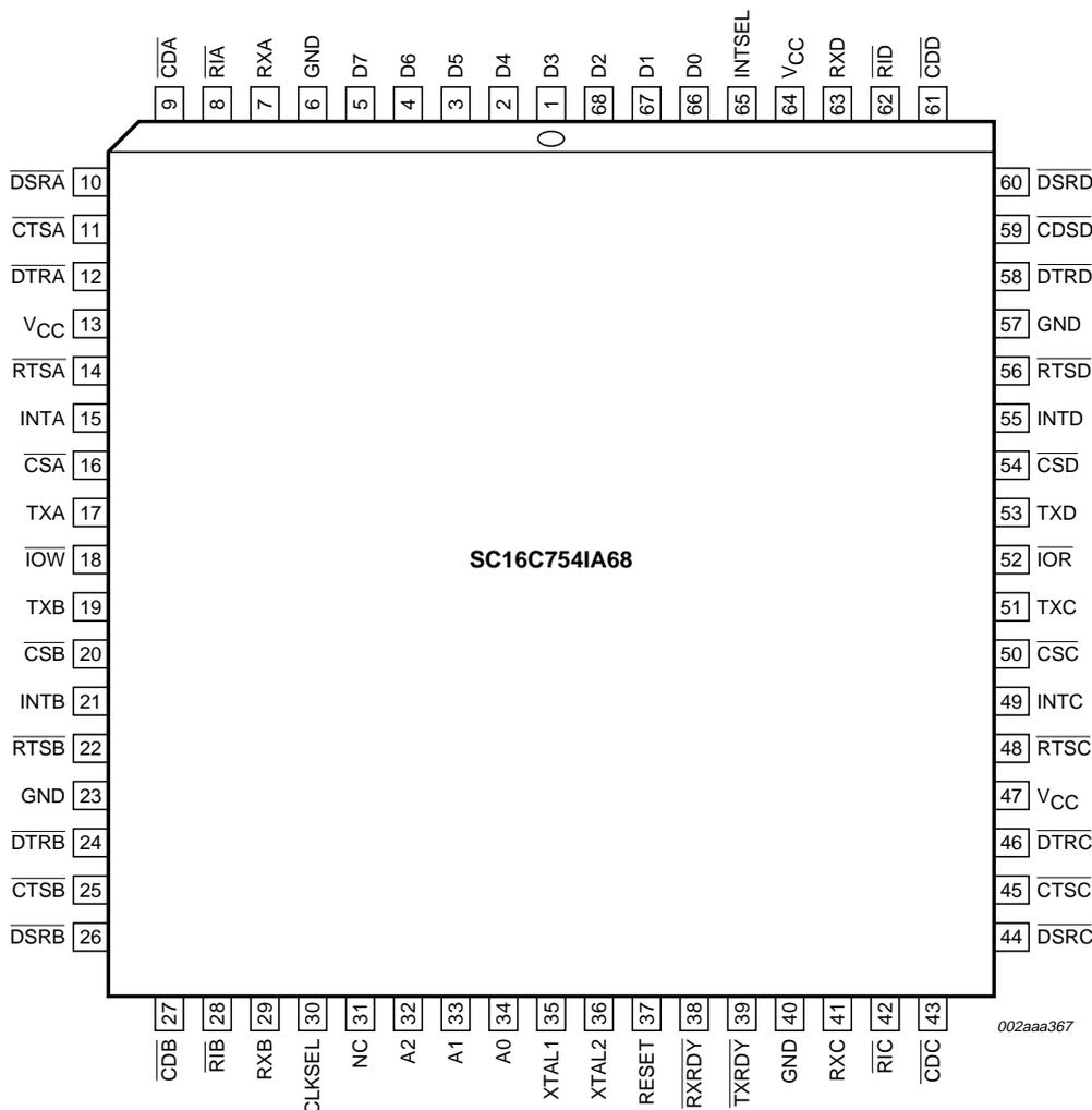
Fig 3. PLCC68 pin configuration.
