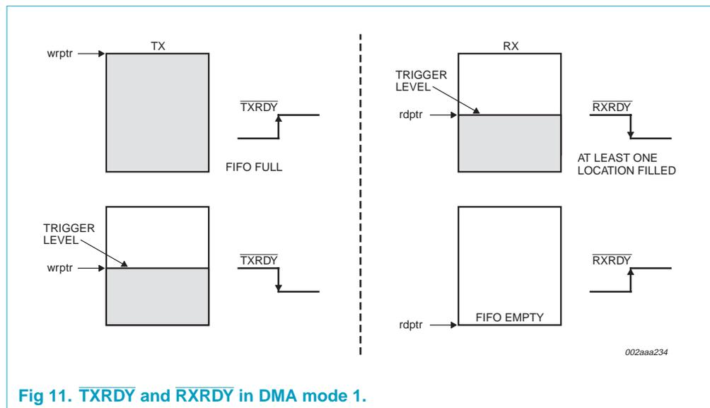
Fig 11.  $\overline{\text{TXRDY}}$  and  $\overline{\text{RXRDY}}$  in DMA mode 1.
