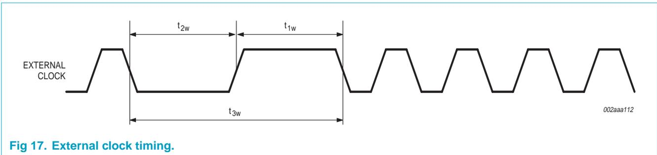
Fig 17. External clock timing.
