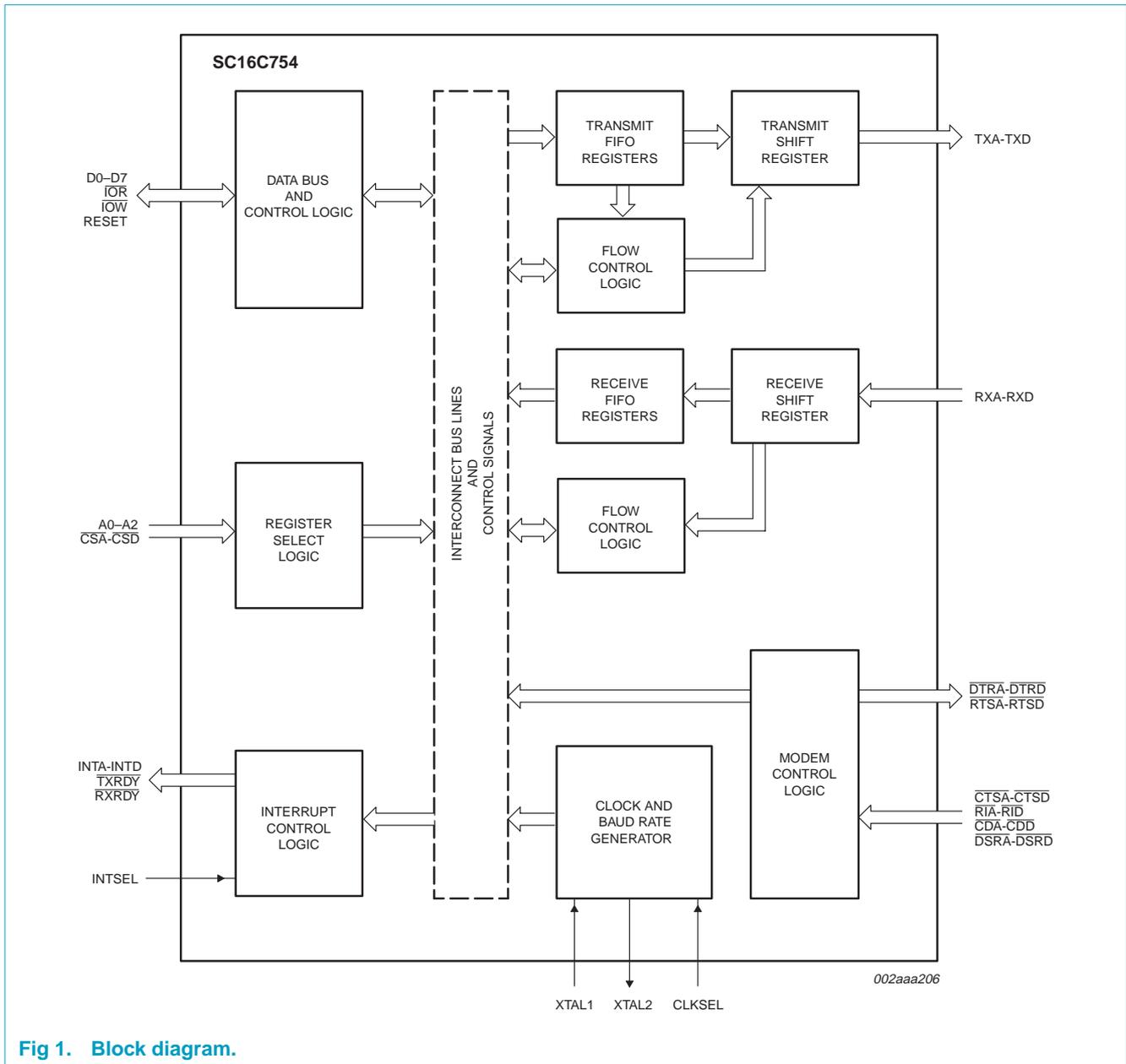
Fig 1. Block diagram.
