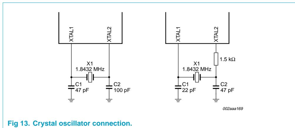
Fig 13. Crystal oscillator connection.
