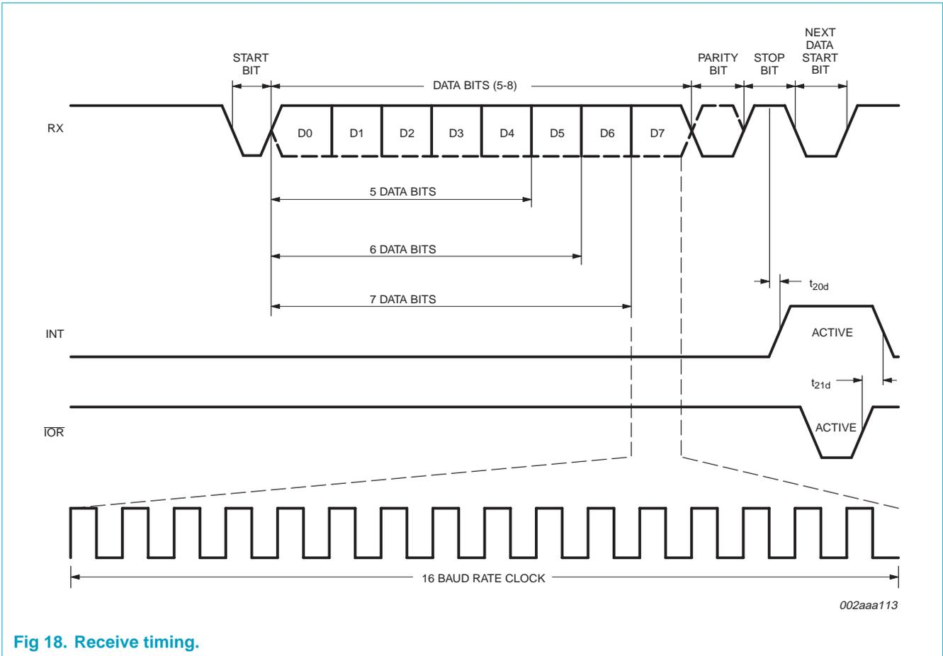
Fig 18. Receive timing.
