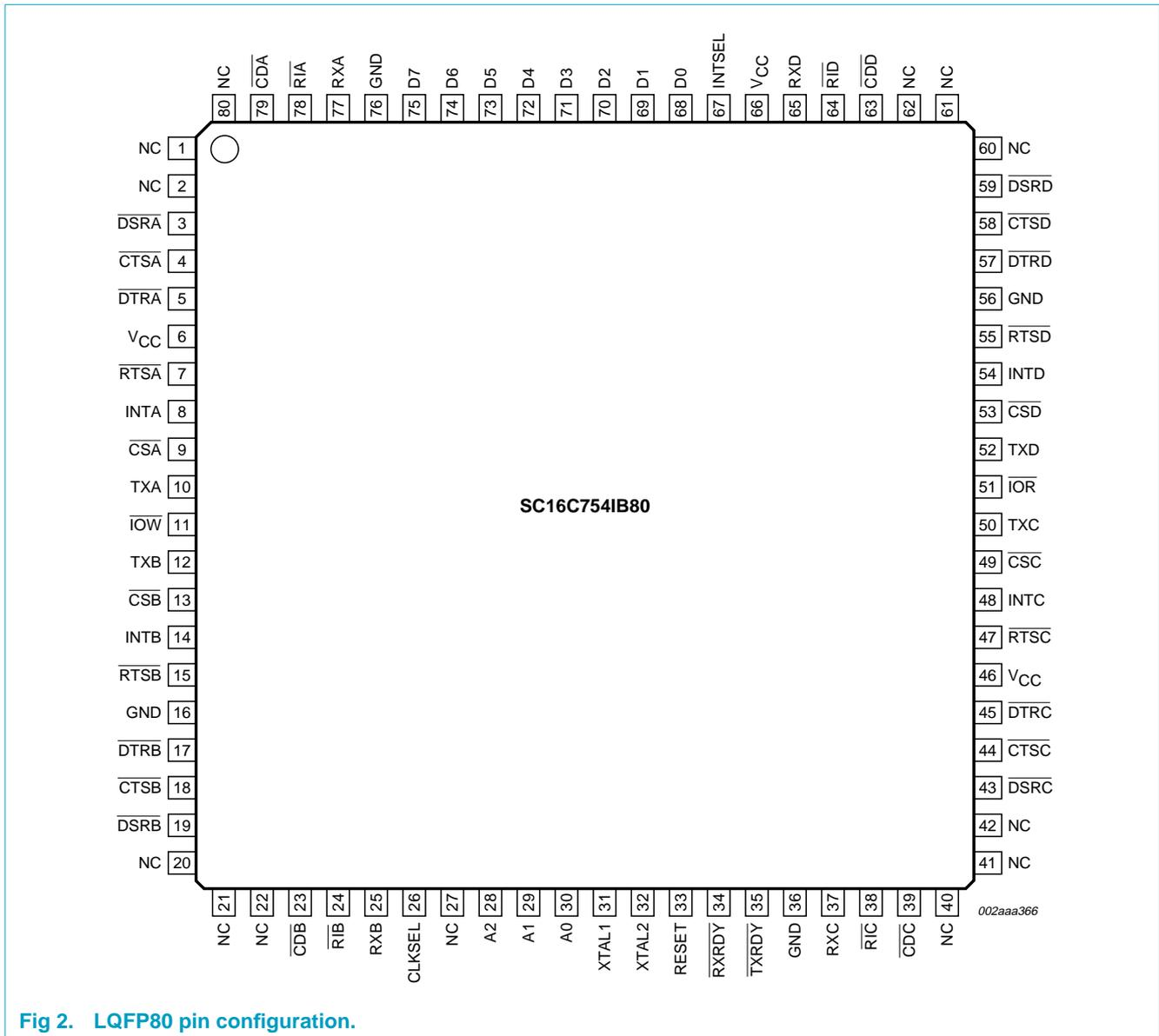
Fig 2. LQFP80 pin configuration.
