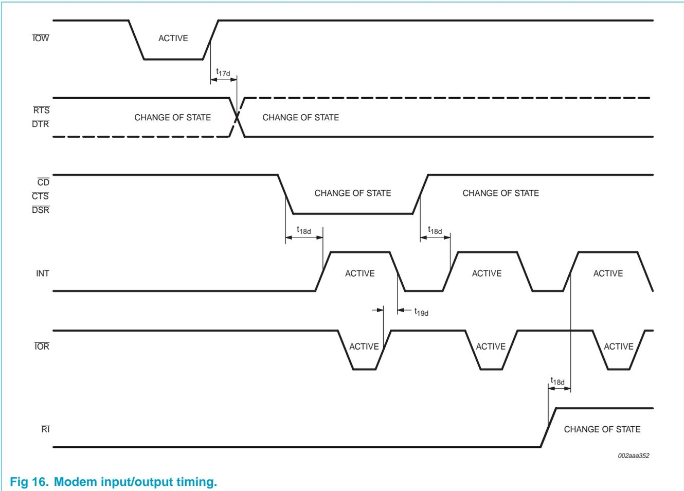
Fig 16. Modem input/output timing.
