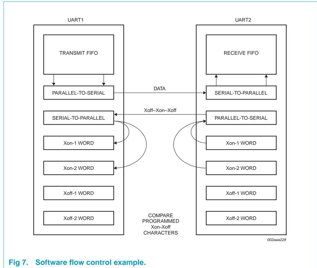
Fig 7. Software flow control example.
