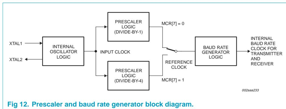
Fig 12. Prescaler and baud rate generator block diagram.
