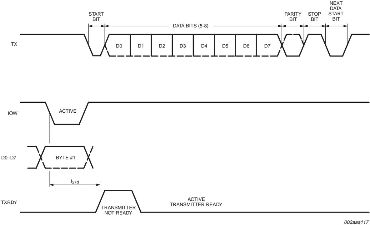
Fig 22. Transmit ready timing in non-FIFO mode.
