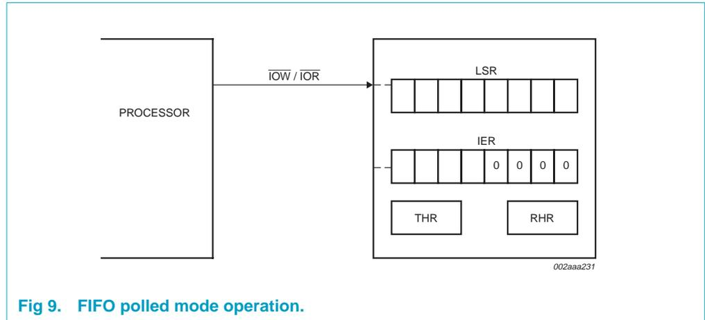
Fig 9. FIFO polled mode operation.
