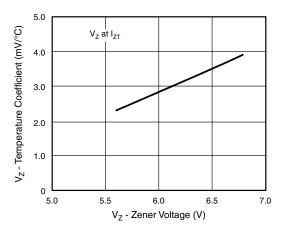
Fig. 4 - Typical temperature Coefficients
