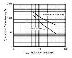
Fig. 6 - Typical Junction Capacitance
