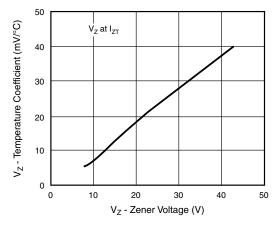
Fig. 5 - Typical Transient Temperature Coefficients
