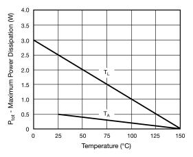
Fig. 1 - Steady State Power Derating
