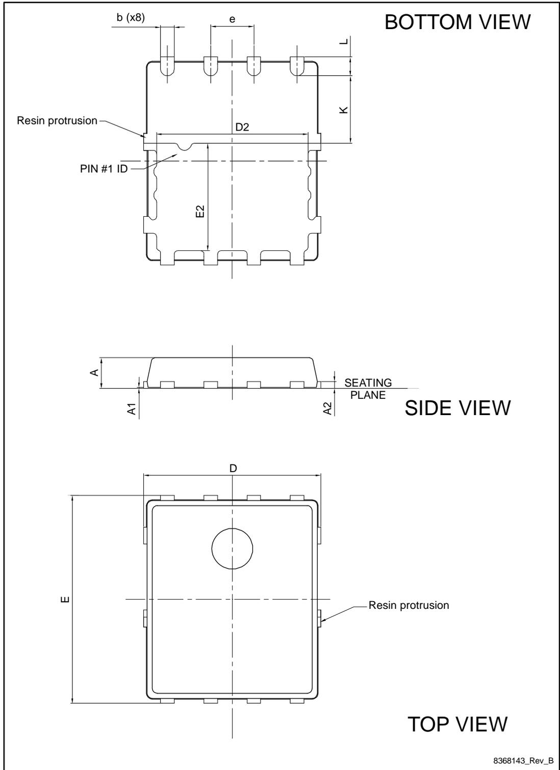
Table 10: PowerFLAT™ 5x6 HV mechanical data
