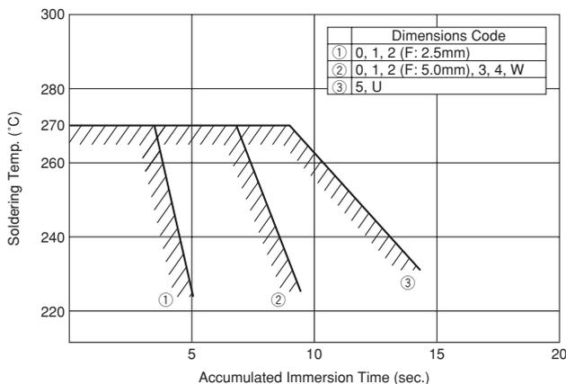
Perform soldering within tolerance range (shaded portion).
