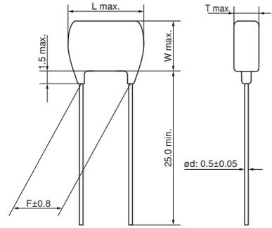
• Lead Wire: Solder Coated CP Wire
