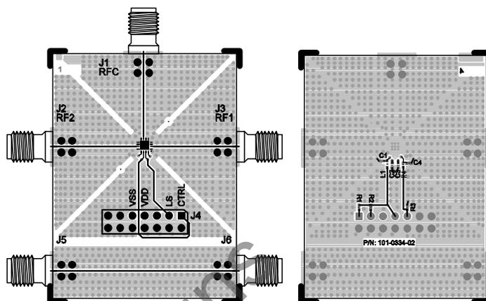
**Figure 17. Evaluation Board Schematic**
