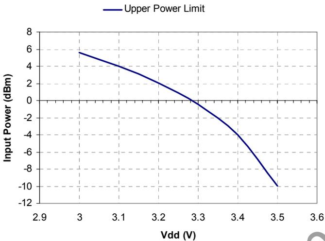
To allow for sustained operation under any load VSWR condition, max power should be kept 6dB lower than max power in 50 Ohm.
