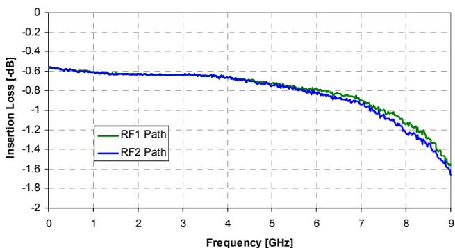
Figure 7. Insertion Loss: RFX @ 3.3 V
