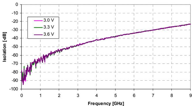
Figure 11. Isolation: RFC to Isolated Port @ 3.3 V
