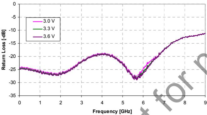
Figure 15. Return Loss at active port @ 3.3 V
