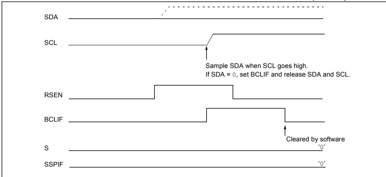
**FIGURE 14-30: BUS COLLISION DURING REPEATED START CONDITION (CASE 2)**
