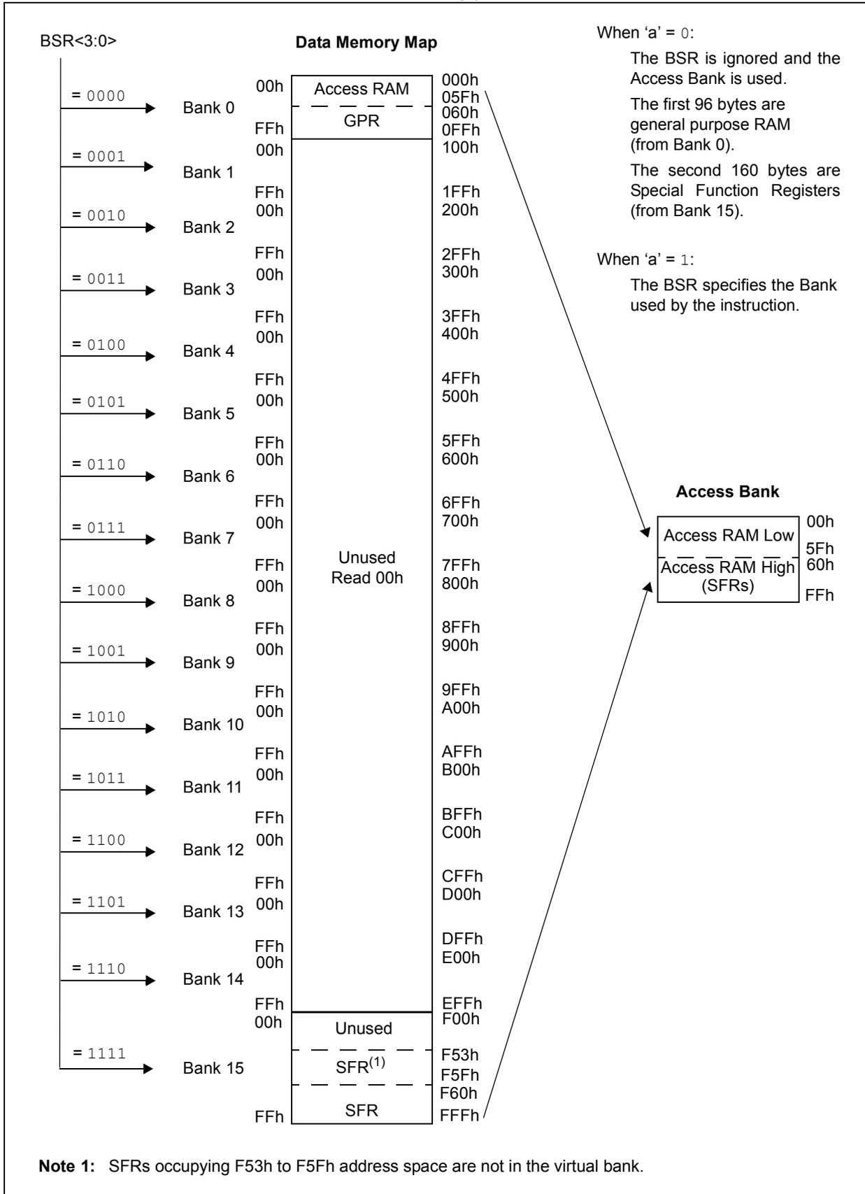
**FIGURE 3-6: DATA MEMORY MAP FOR PIC18(L)F14K22 DEVICES**
