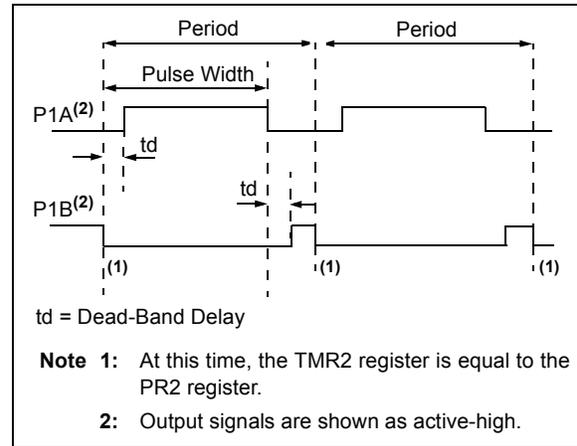
**FIGURE 13-7: EXAMPLE OF HALF-BRIDGE APPLICATIONS**
