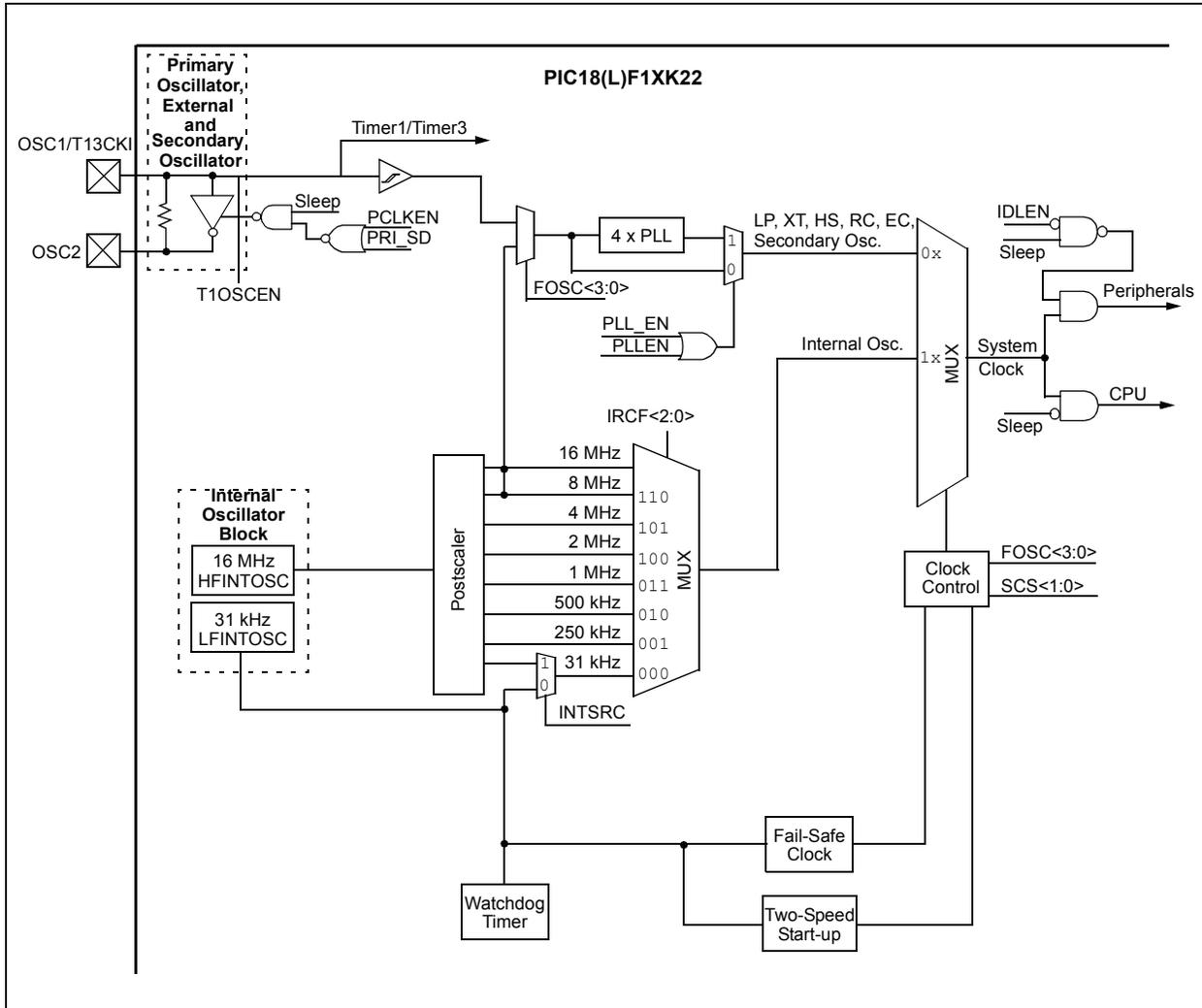
**Note:** If using a low-frequency external oscillator and want to multiple it by 4 via PLL, the ideal input frequency is from 4 MHz to 16 MHz.
