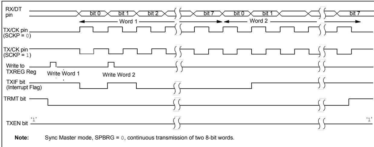
**FIGURE 15-11: SYNCHRONOUS TRANSMISSION (THROUGH TXEN)**
