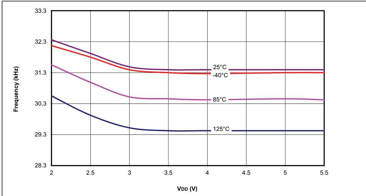
FIGURE 26-26: PIC18F1XK22 TYPICAL LF-INTOSC FREQUENCY (MAX./MIN. = 31.25 kHz  $\pm$  15%)
