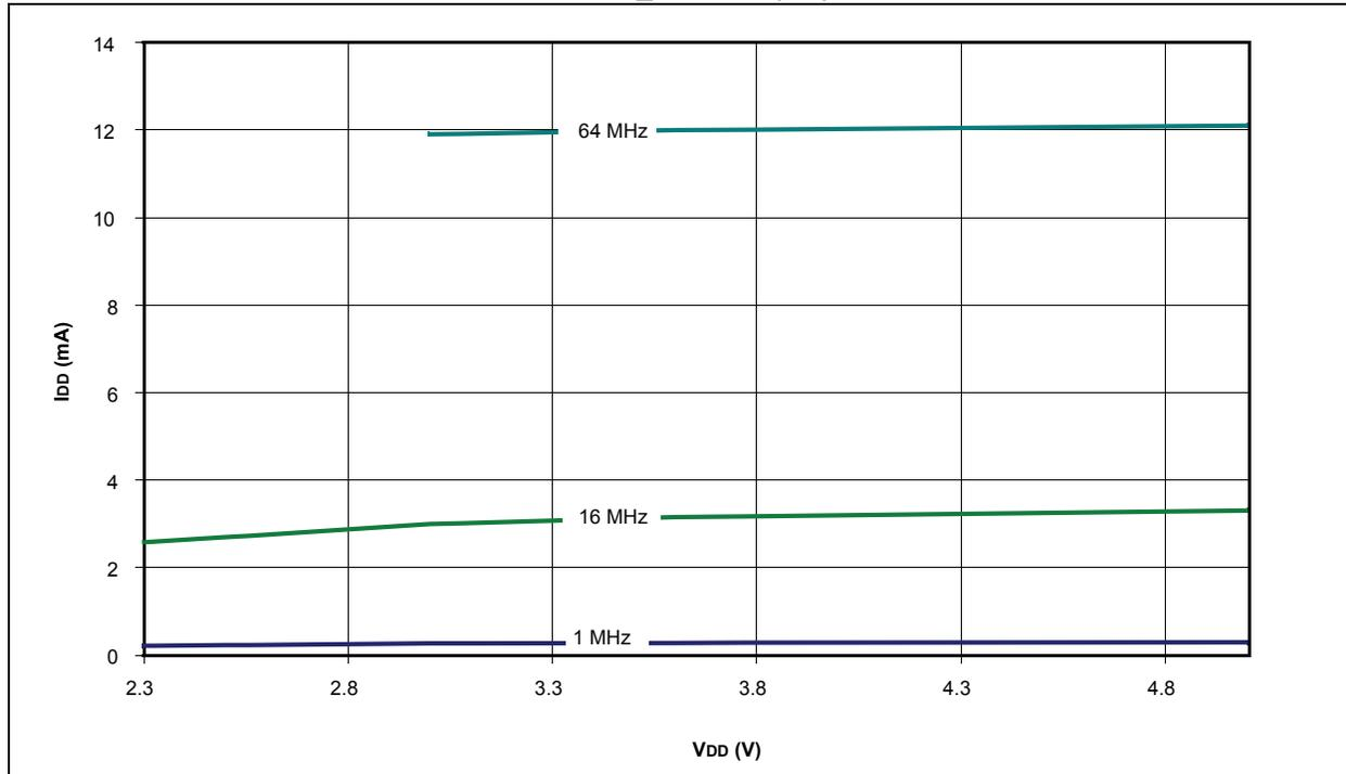
FIGURE 26-20: PIC18F1XK22 TYPICAL PRI\_RUN I<sub>DD</sub> (HS + PLL)
