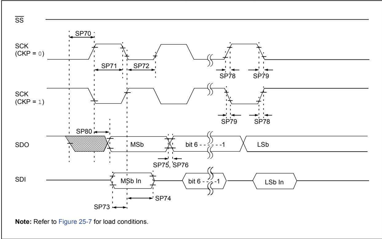
**FIGURE 25-18: SPI MASTER MODE TIMING (CKE = 1, SMP = 1)**
