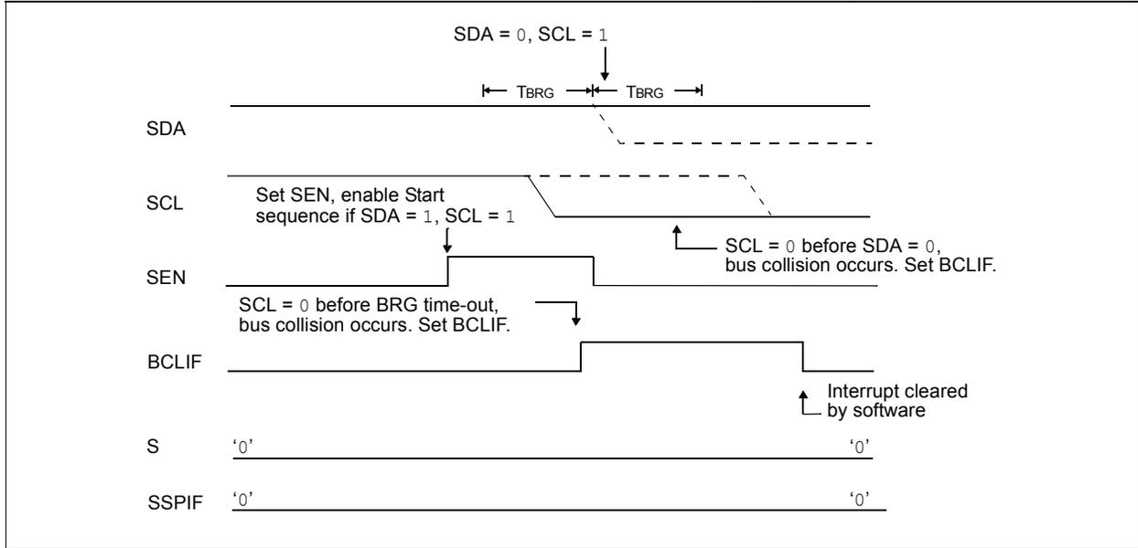
**FIGURE 14-28: BRG RESET DUE TO SDA ARBITRATION DURING START CONDITION**
