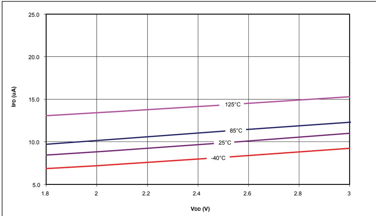
**FIGURE 26-6: PIC18LF1XK22 I<sub>COMP</sub> – TYPICAL I<sub>PD</sub> FOR COMPARATOR IN HIGH-POWER MODE**
