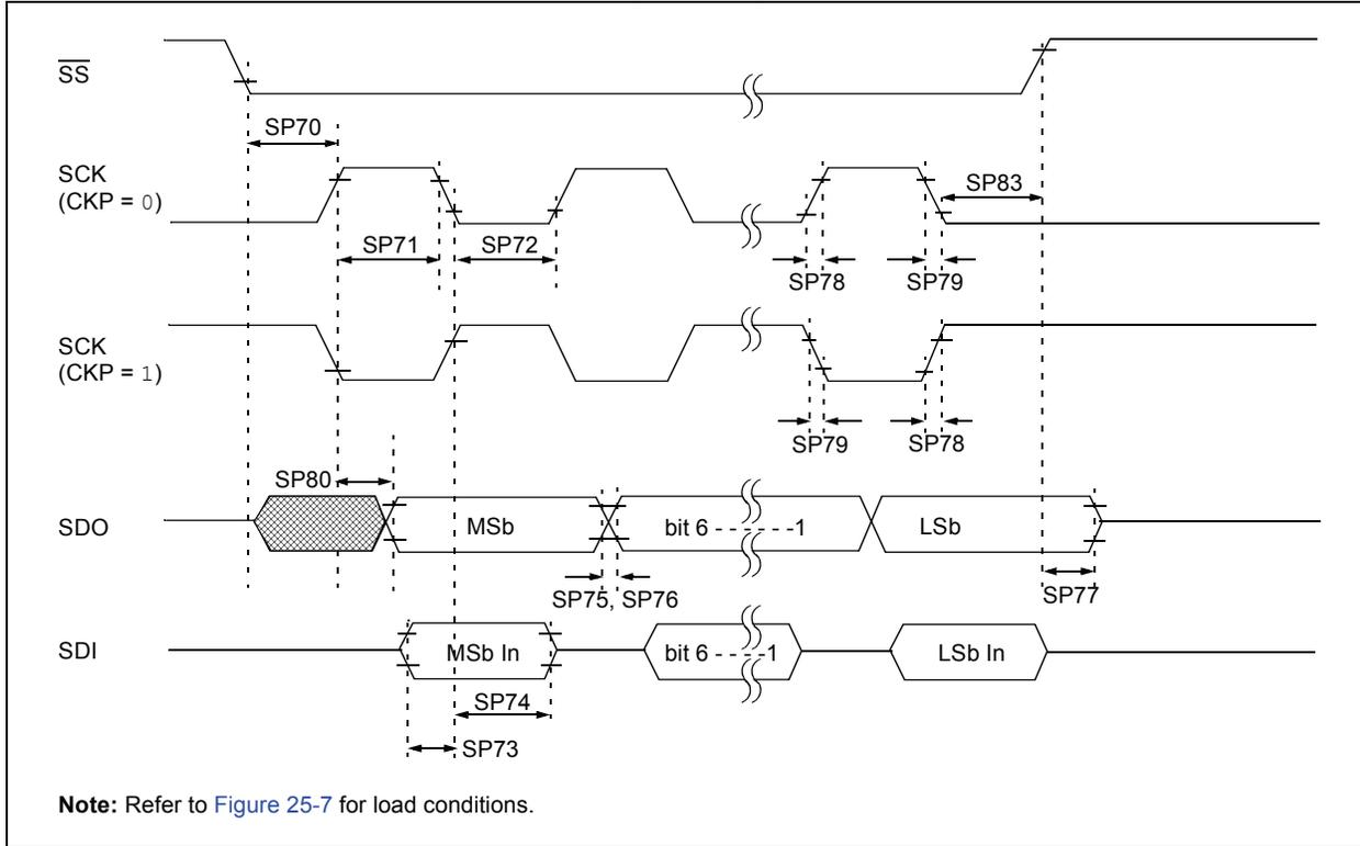
**FIGURE 25-20: SPI SLAVE MODE TIMING (CKE = 1)**
