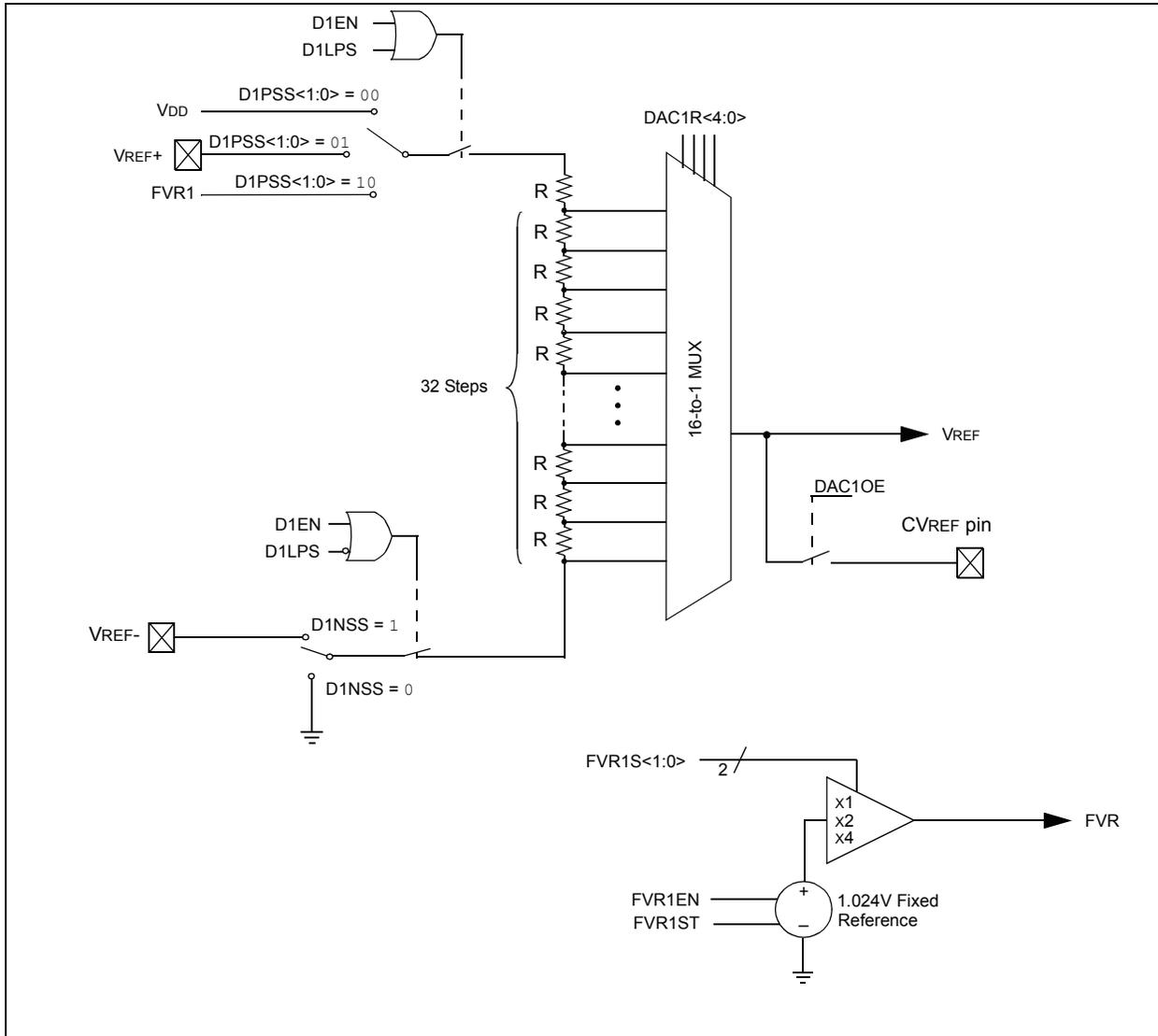
**FIGURE 20-2: VOLTAGE REFERENCE OUTPUT BUFFER EXAMPLE**
