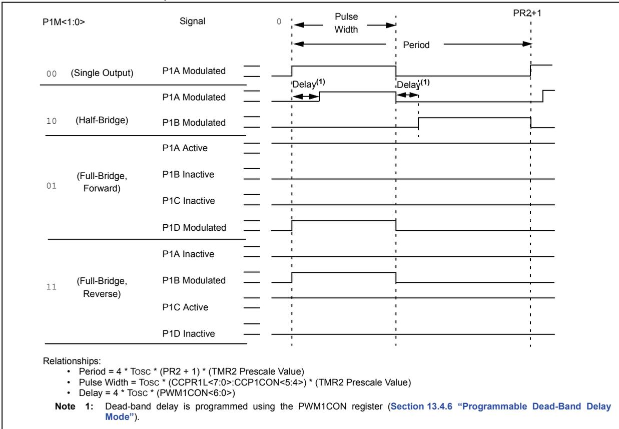
**FIGURE 13-5: EXAMPLE ENHANCED PWM OUTPUT RELATIONSHIPS (ACTIVE-LOW STATE)**
