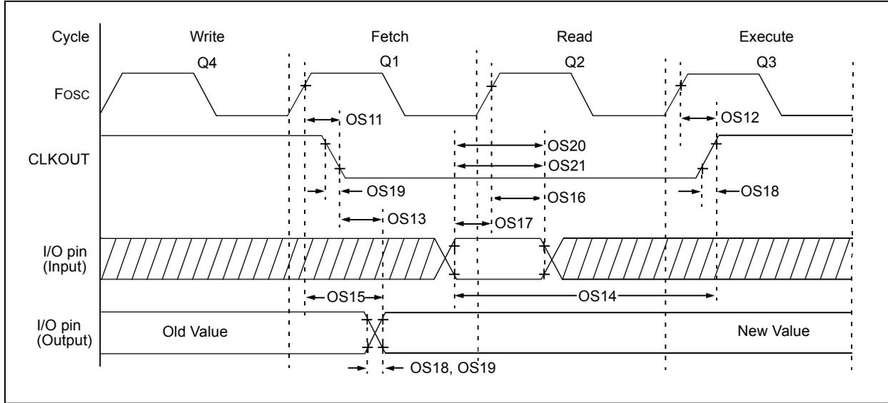
**TABLE 25-4: CLKOUT AND I/O TIMING PARAMETERS**
