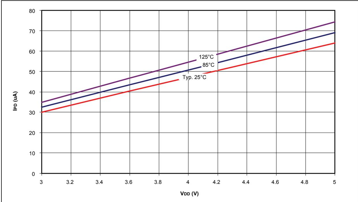
**FIGURE 26-14: PIC18F1XK22 TYPICAL  $I_{PD}$  FOR COMPARATOR VOLTAGE REFERENCE**
