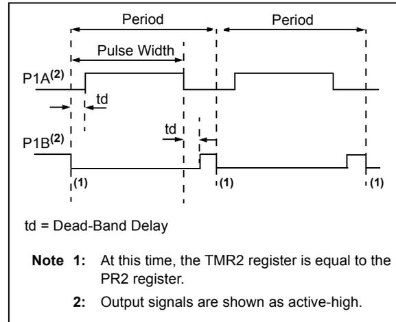
**FIGURE 13-15: EXAMPLE OF HALF-BRIDGE APPLICATIONS**
