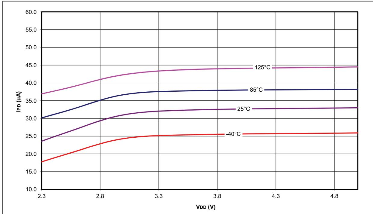
FIGURE 26-16: PIC18F1XK22 I<sub>COMP</sub> – TYPICAL I<sub>PD</sub> FOR COMPARATOR IN HIGH-POWER MODE
