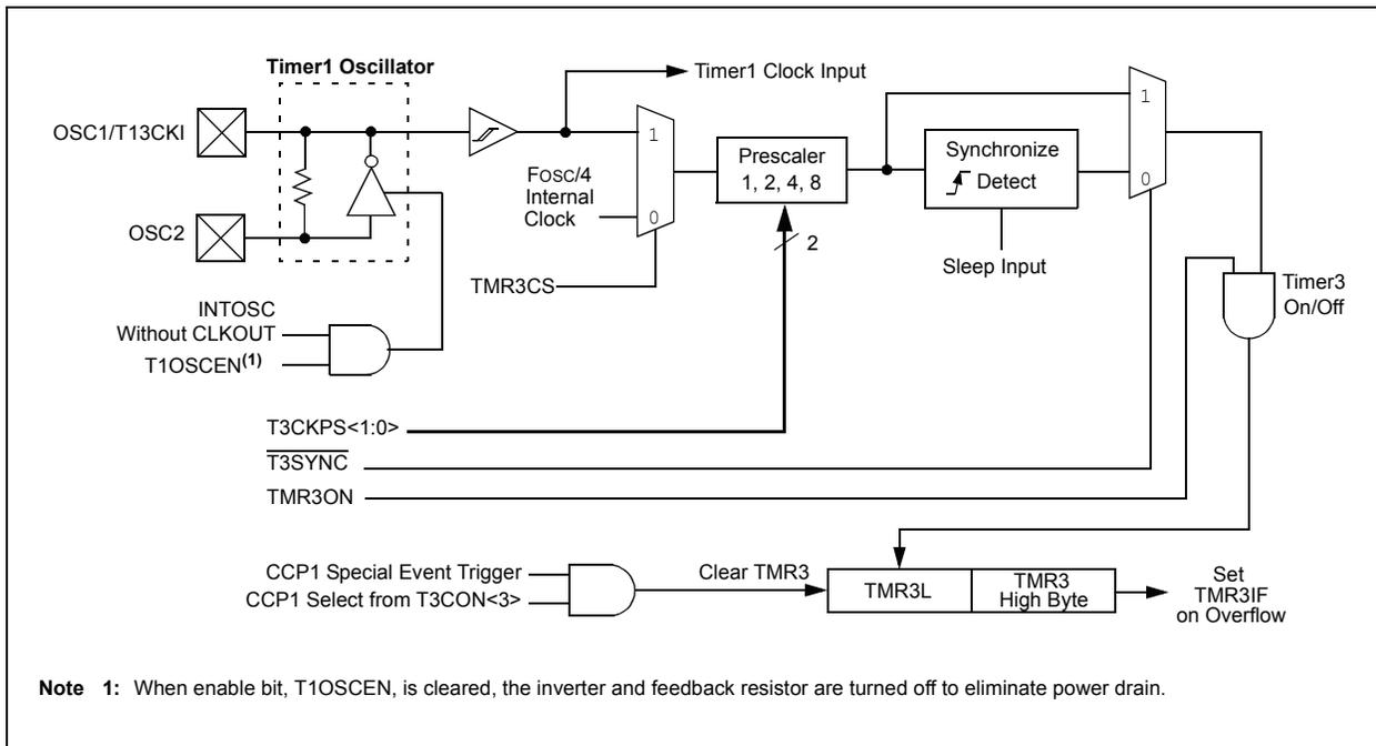
**FIGURE 12-2: TIMER3 BLOCK DIAGRAM (16-BIT READ/WRITE MODE)**
