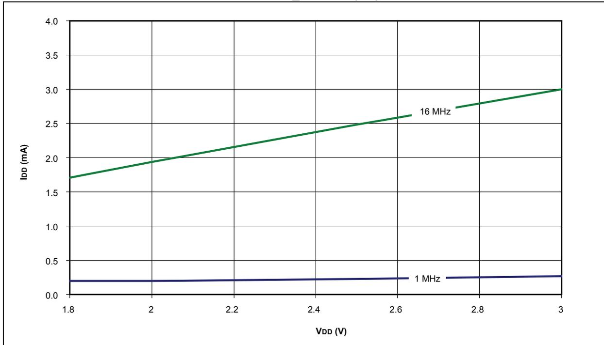
**FIGURE 26-10: PIC18LF1XK22 TYPICAL PRI\_RUN I<sub>DD</sub> (HS + PLL)**
