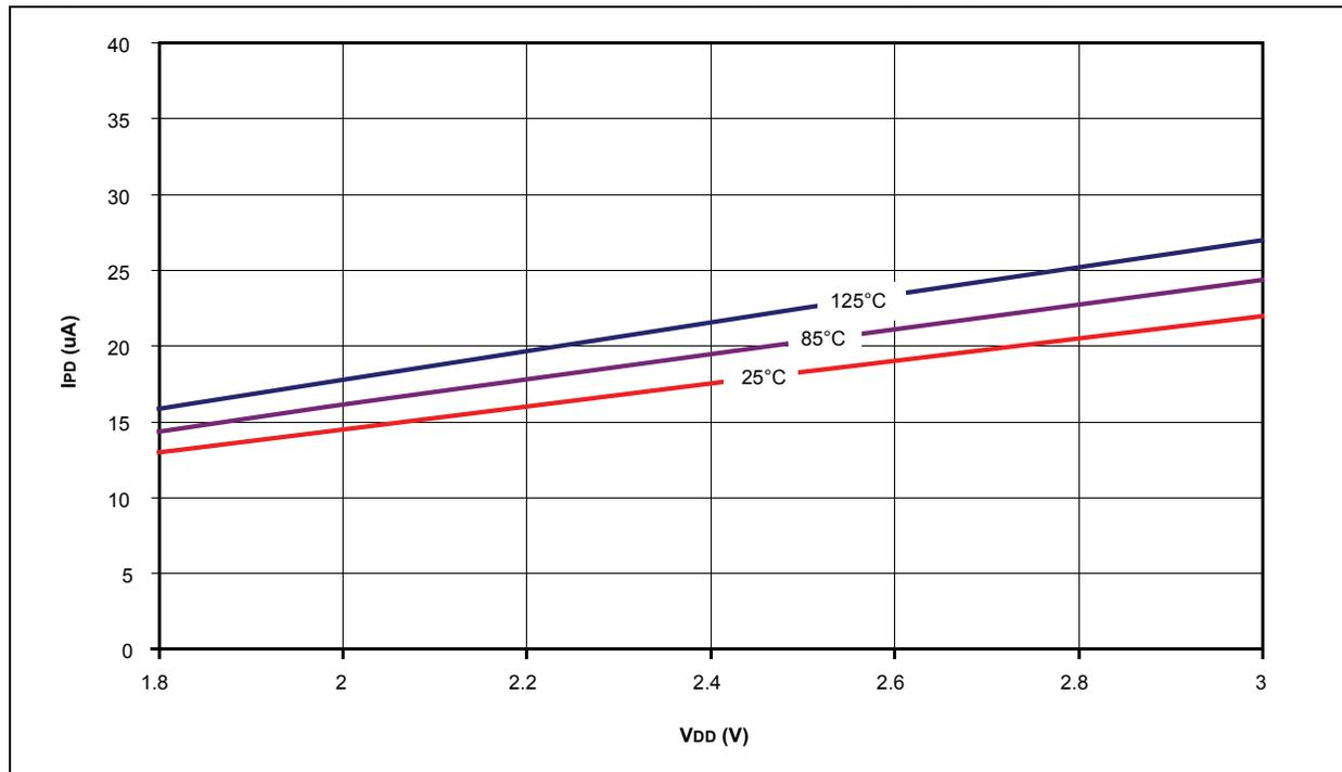
**FIGURE 26-5: PIC18LF1XK22 I<sub>COMP</sub> – TYPICAL I<sub>PD</sub> FOR COMPARATOR IN LOW-POWER MODE**
