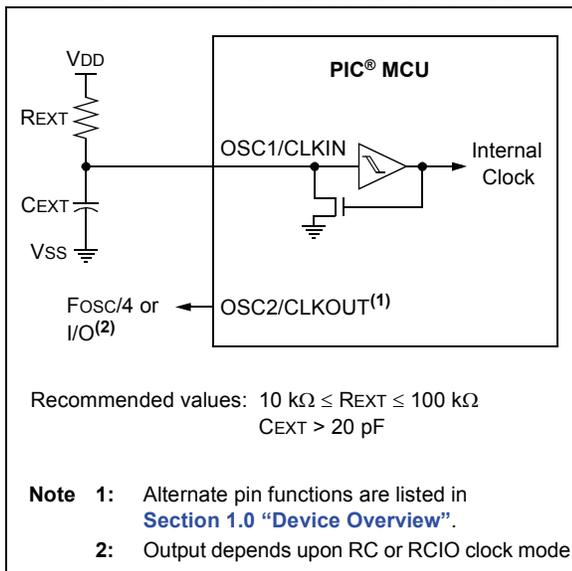
The RC oscillator frequency is a function of the supply voltage, the resistor  $R_{EXT}$ , the capacitor  $C_{EXT}$  and the operating temperature. Other factors affecting the oscillator frequency are:
