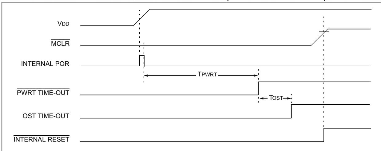
**FIGURE 21-6: SLOW RISE TIME ( $\overline{\text{MCLR}}$  TIED TO  $V_{DD}$ ,  $V_{DD}$  RISE  $>$   $T_{PWRT}$ )**
