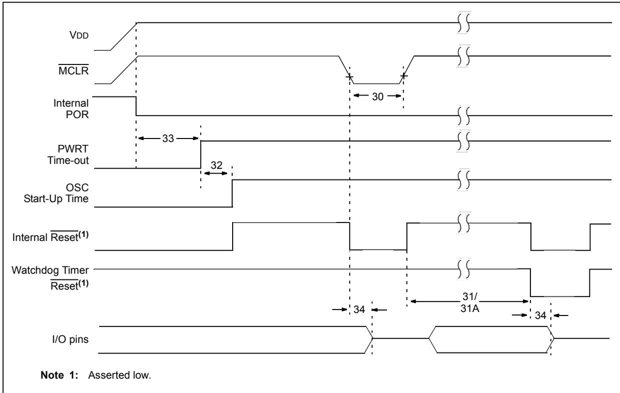
**FIGURE 25-11: BROWN-OUT RESET TIMING AND CHARACTERISTICS**
