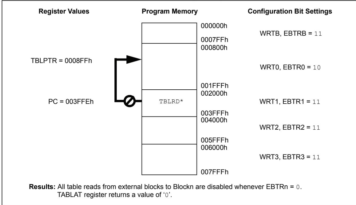
**FIGURE 22-5: EXTERNAL BLOCK TABLE READ (EBTRn) ALLOWED**
