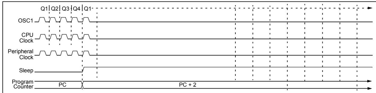
**FIGURE 18-2: TRANSITION TIMING FOR WAKE FROM SLEEP (HSPLL)**
