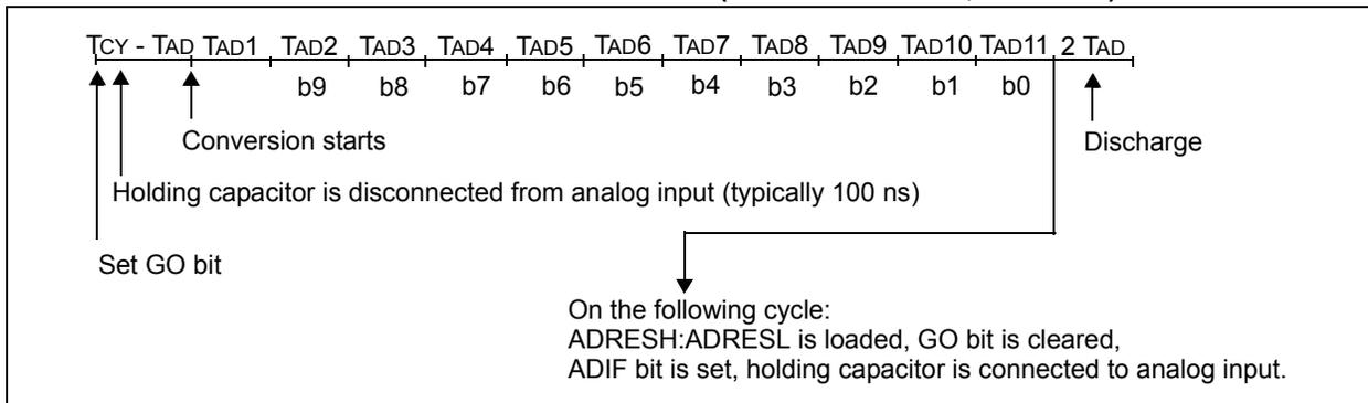
**FIGURE 16-4: A/D CONVERSION TAD CYCLES (`ACQT<2:0> = 010, TACQ = 4 TAD`)**
