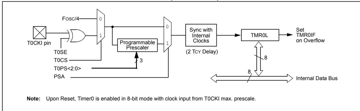
**FIGURE 9-2: TIMER0 BLOCK DIAGRAM (16-BIT MODE)**
