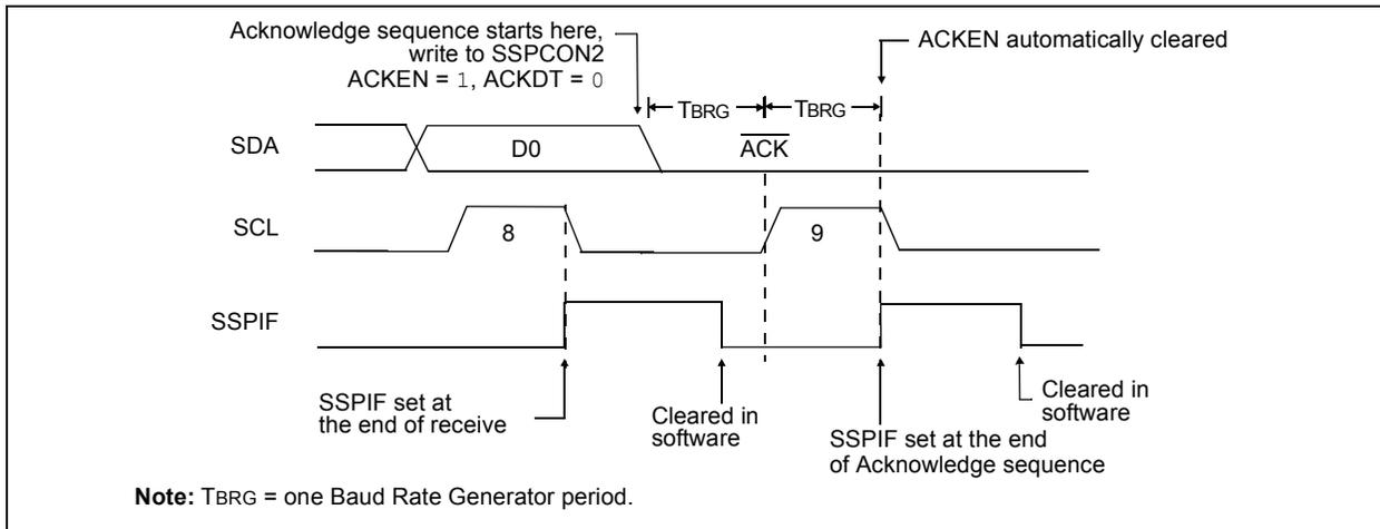
**FIGURE 14-24: STOP CONDITION RECEIVE OR TRANSMIT MODE**
