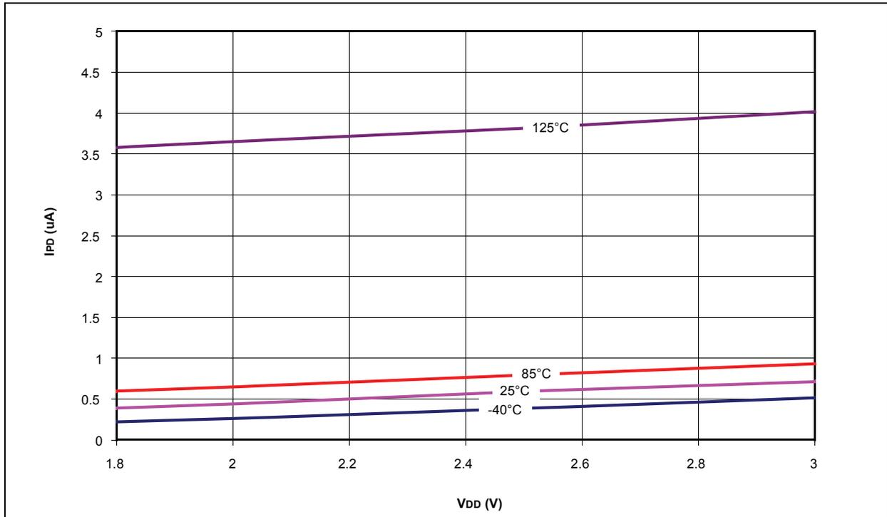
FIGURE 26-2: PIC18LF1XK22 TYPICAL IPD FOR WATCHDOG TIMER
