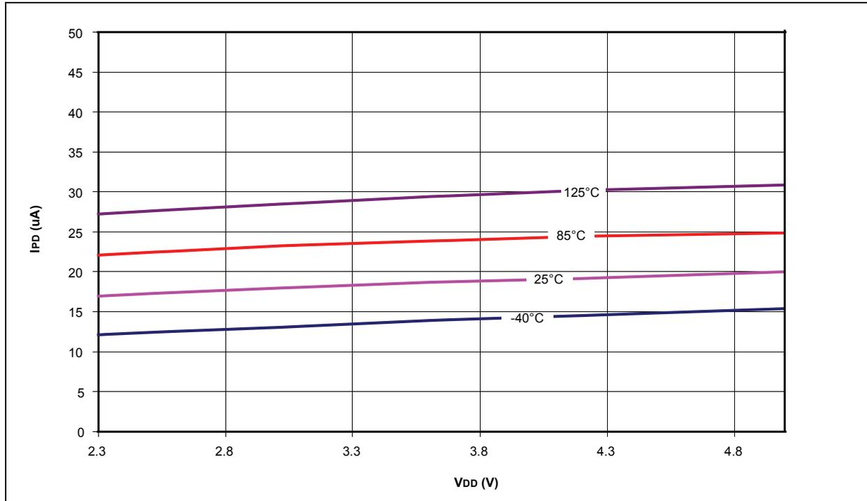
FIGURE 26-12: PIC18F1XK22 TYPICAL I<sub>PD</sub> FOR WATCHDOG TIMER
