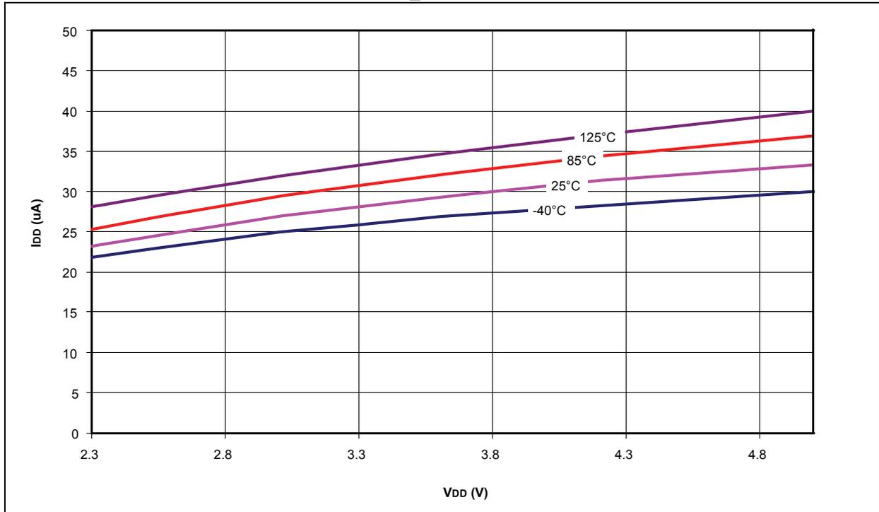
FIGURE 26-18: PIC18F1XK22 TYPICAL RC\_RUN I<sub>DD</sub>
