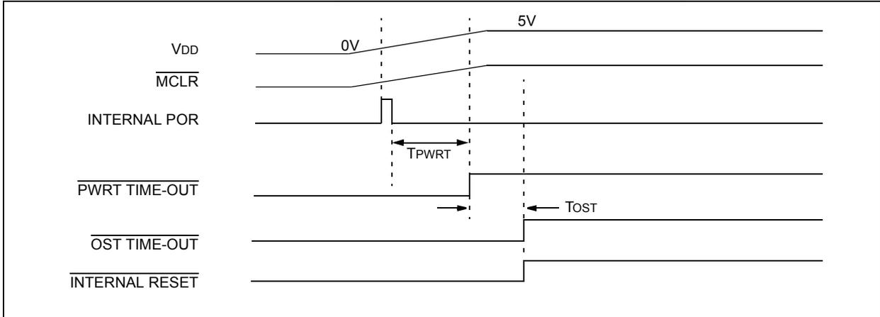
**FIGURE 21-7: TIME-OUT SEQUENCE ON POR W/PLL ENABLED ( $\overline{\text{MCLR}}$  TIED TO  $V_{DD}$ )**
