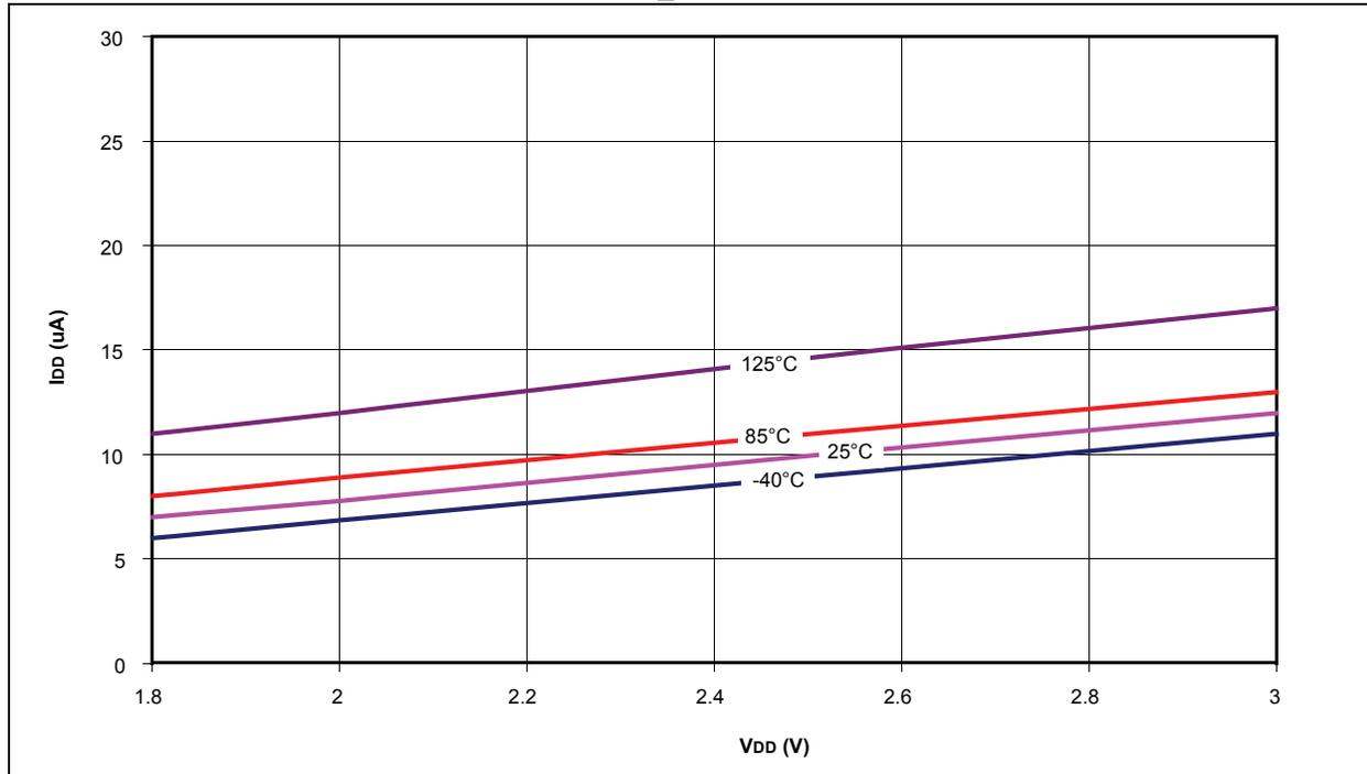
FIGURE 26-8: PIC18LF1XK22 TYPICAL RC\_RUN I<sub>DD</sub>
