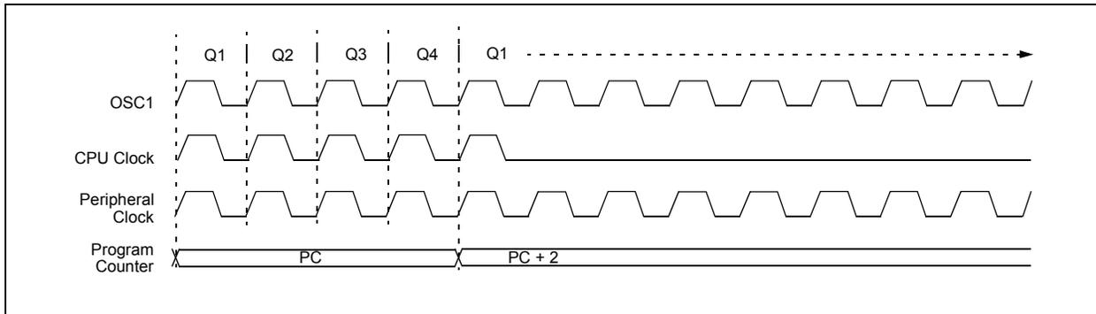
**FIGURE 18-4: TRANSITION TIMING FOR WAKE FROM IDLE TO RUN MODE**
