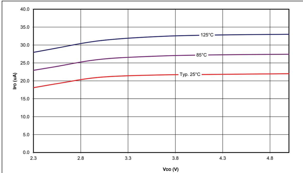
**FIGURE 26-13: PIC18F1XK22 TYPICAL  $I_{PD}$  FOR BROWN-OUT RESET**
