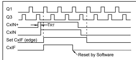
**FIGURE 17-5: COMPARATOR INTERRUPT TIMING WITH CMxCON0 READ**
