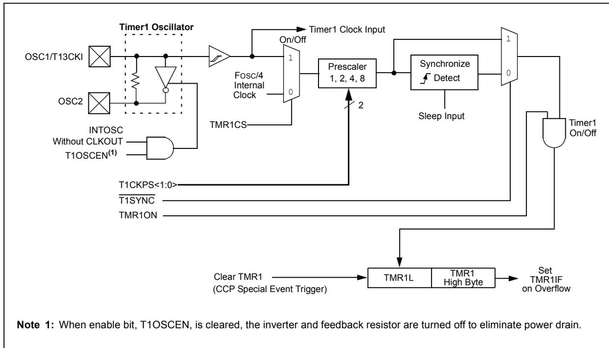
**FIGURE 10-2: TIMER1 BLOCK DIAGRAM (16-BIT READ/WRITE MODE)**
