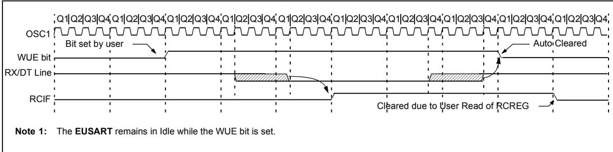
**FIGURE 15-8: AUTO-WAKE-UP BIT (WUE) TIMINGS DURING SLEEP**
