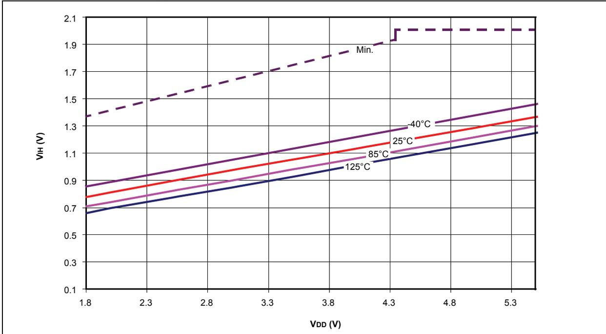
**FIGURE 26-22: PIC18(L)F1XK22 SCHMITT TRIGGER BUFFER TYPICAL  $V_{IH}$**
