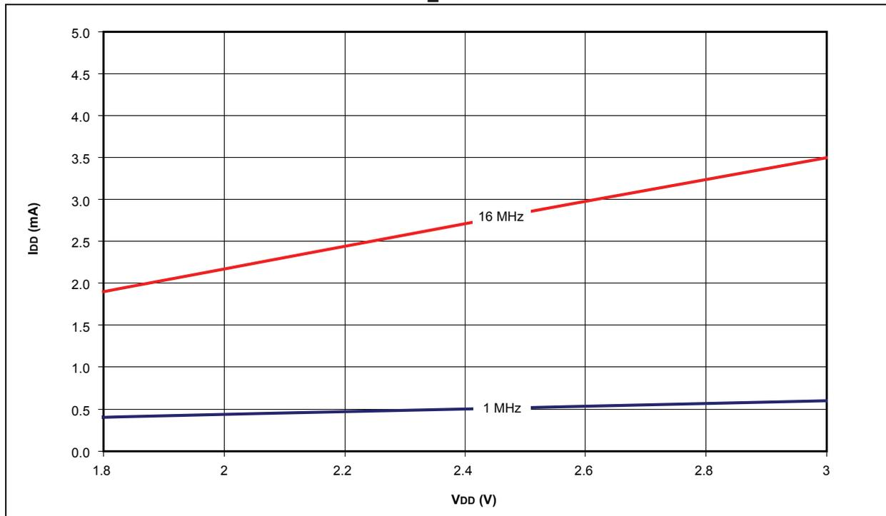
**FIGURE 26-9: PIC18LF1XK22 TYPICAL PRI\_RUN I<sub>DD</sub> (EC)**
