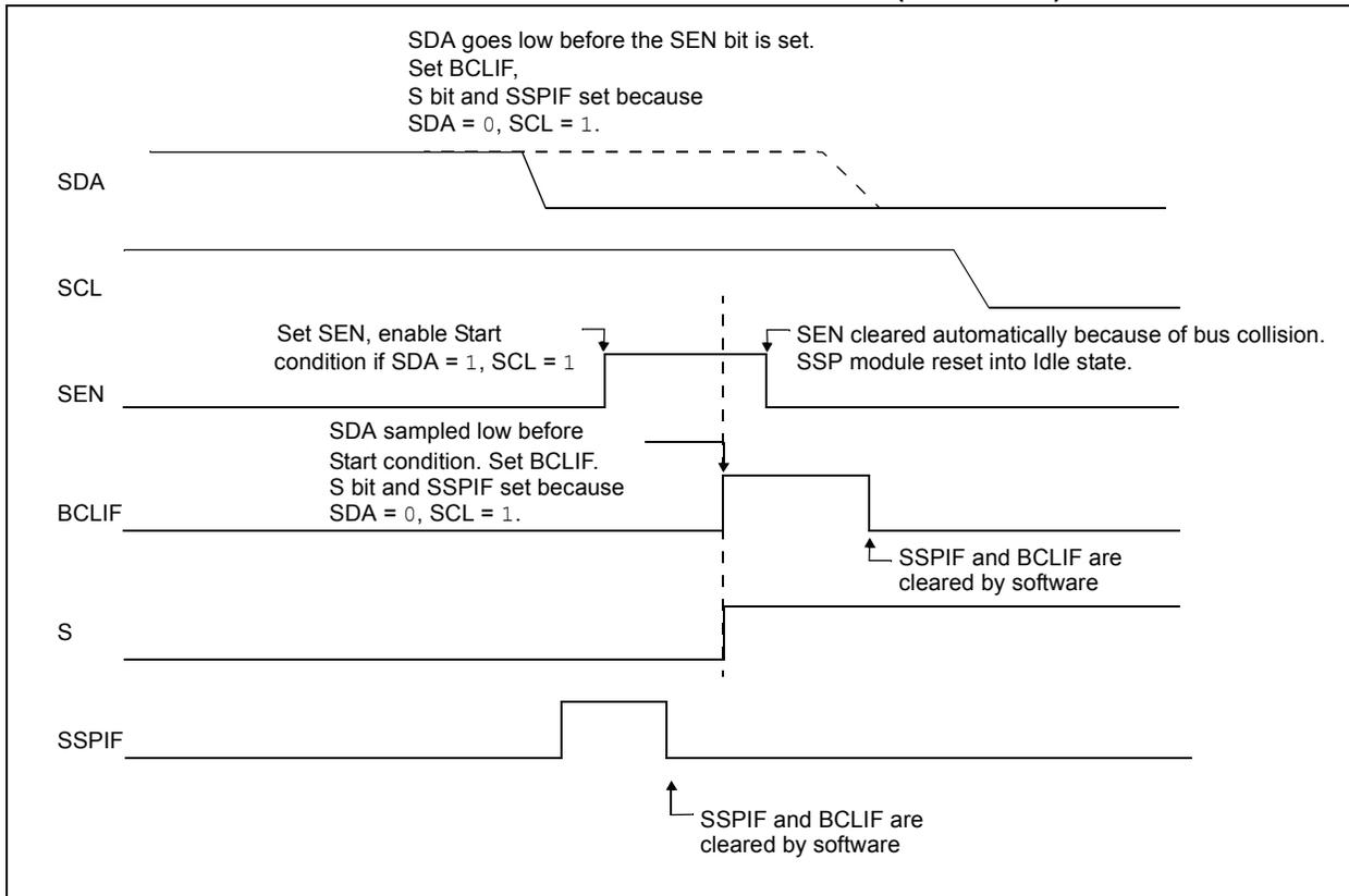
**FIGURE 14-27: BUS COLLISION DURING START CONDITION (SCL = 0)**
