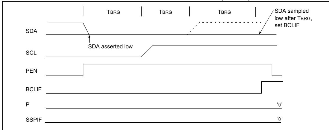
**FIGURE 14-32: BUS COLLISION DURING A STOP CONDITION (CASE 2)**
