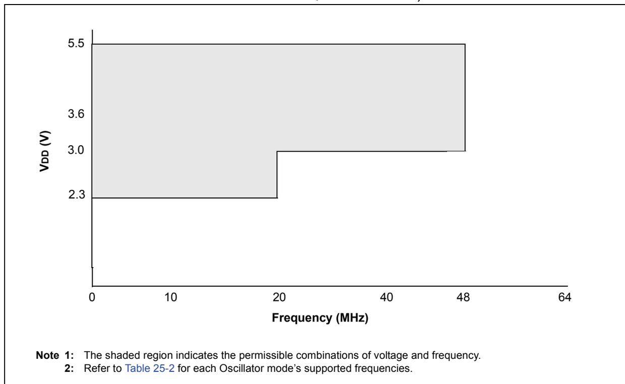
**FIGURE 25-3: PIC18LF1XK22 VOLTAGE FREQUENCY GRAPH,  $-40^{\circ}\text{C} \leq T_A \leq +85^{\circ}\text{C}$**
