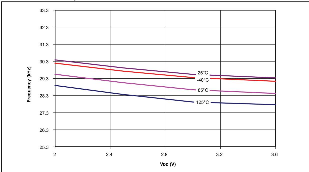
**FIGURE 26-28: PIC18LF1XK22 TYPICAL LF-INTOSC FREQUENCY (MAX./MIN. = 31.25 kHz  $\pm$  15%)**
