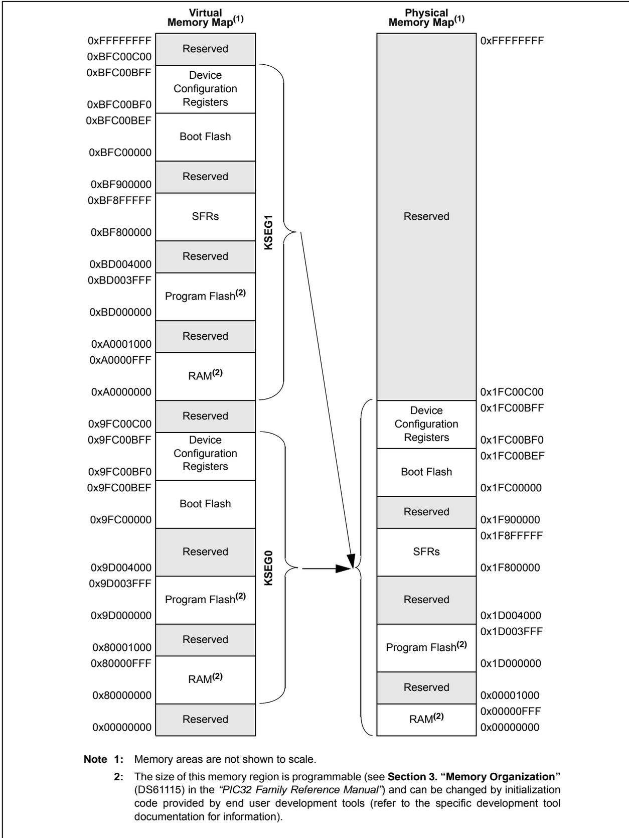
**FIGURE 4-2: MEMORY MAP ON RESET FOR PIC32MX12X/22X DEVICES**
