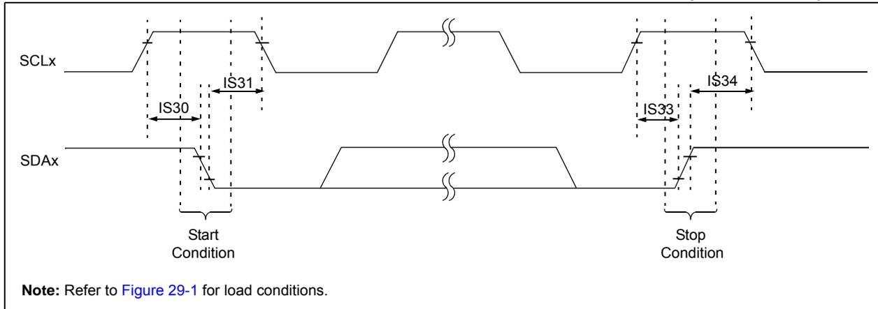
**FIGURE 29-17: I2Cx BUS DATA TIMING CHARACTERISTICS (SLAVE MODE)**
