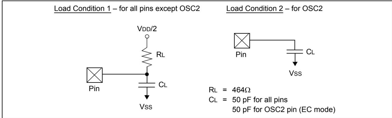
**TABLE 29-14: CAPACITIVE LOADING REQUIREMENTS ON OUTPUT PINS**
