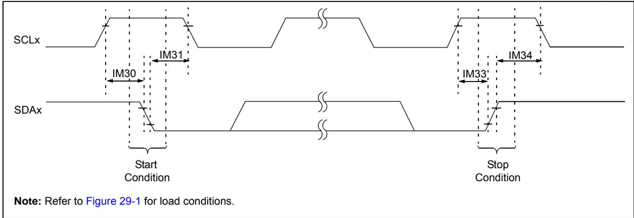
**FIGURE 29-15: I2Cx BUS DATA TIMING CHARACTERISTICS (MASTER MODE)**
