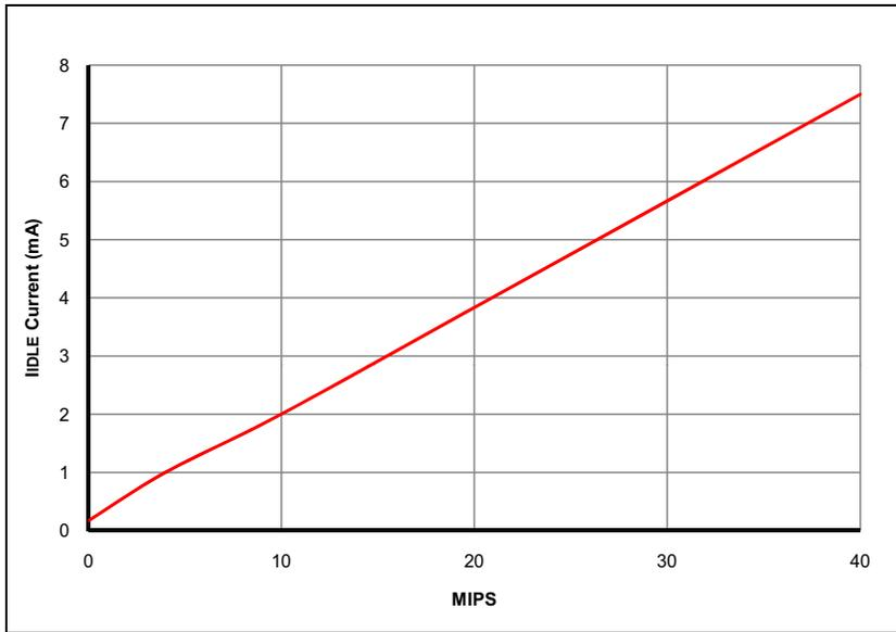
**FIGURE 30-4: TYPICAL I<sub>DD</sub> CURRENT @ V<sub>DD</sub> = 3.3V**
