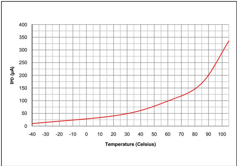
**FIGURE 30-5: TYPICAL I<sub>IDLE</sub> CURRENT @ V<sub>DD</sub> = 3.3V**
