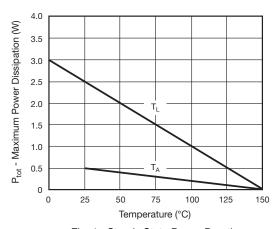
Fig. 1 - Steady State Power Durating
