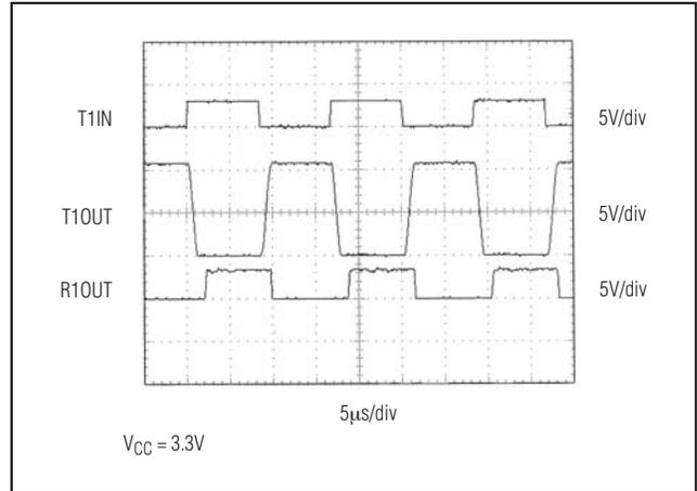
Figure 6. MAX3241 Loopback Test Result at 120kbps
