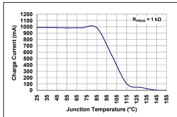
**FIGURE 2-12:** Charge Current ( $I_{OUT}$ ) vs. Junction Temperature ( $T_J$ ).
