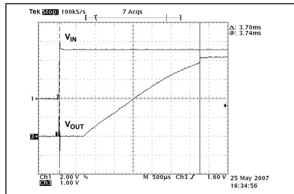
**FIGURE 2-24:**  $V_{USB}$  Start Delay (USB = Low).
