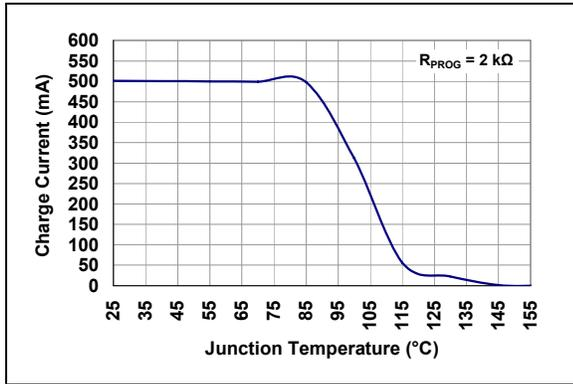
**FIGURE 2-13:** Charge Current ( $I_{OUT}$ ) vs. Junction Temperature ( $T_J$ ).
