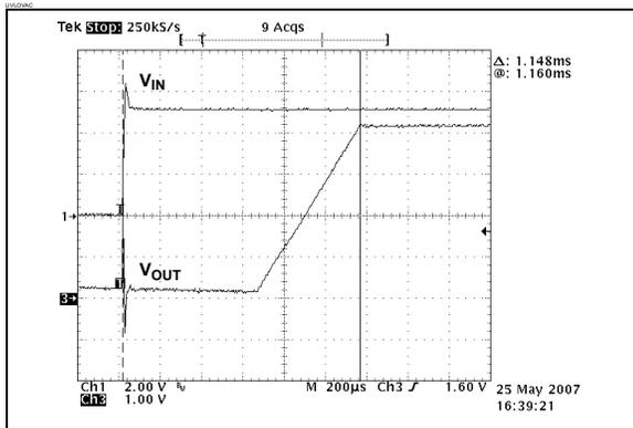
**FIGURE 2-25:**  $V_{USB}$  Start Delay (USB = High)
