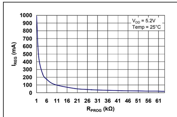
**FIGURE 2-6:** Charge Current ( $I_{OUT}$ ) vs. Programming Resistor ( $R_{PROG}$ ).
