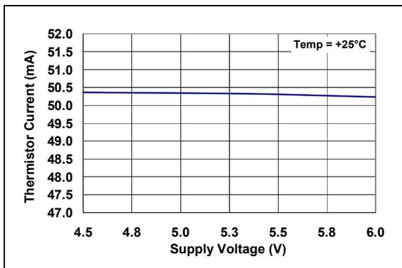
**FIGURE 2-15:** Thermistor Current ( $I_{THERM}$ ) vs. Supply Voltage ( $V_{DD}$ ).
