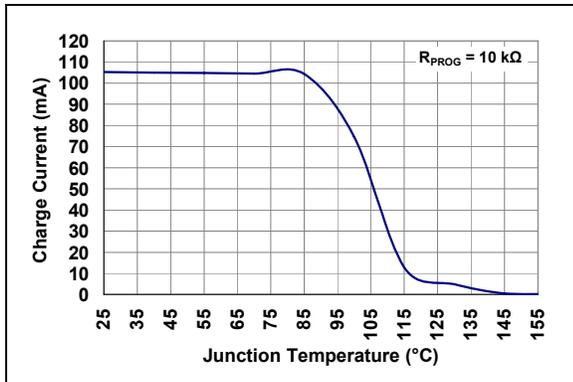
**FIGURE 2-14:** Charge Current ( $I_{OUT}$ ) vs. Junction Temperature ( $T_J$ ).
