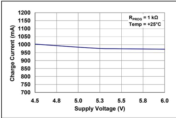
**FIGURE 2-7:** Charge Current ( $I_{OUT}$ ) vs. Supply Voltage ( $V_{DD}$ ).
