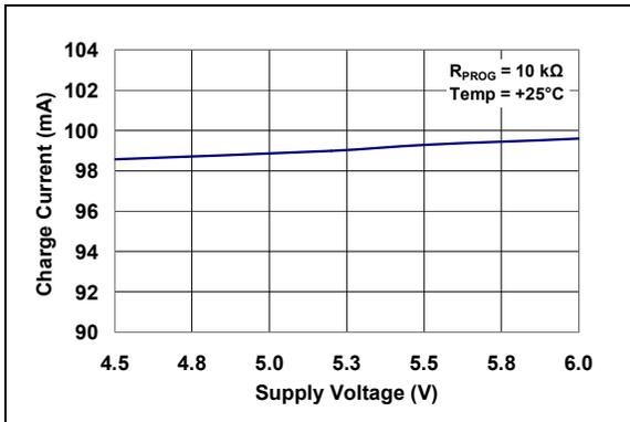
**FIGURE 2-8:** Charge Current ( $I_{OUT}$ ) vs. Supply Voltage ( $V_{DD}$ ).
