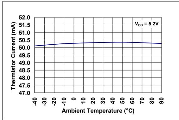
**FIGURE 2-16:** Thermistor Current ( $I_{THERM}$ ) vs. Ambient Temperature ( $T_A$ ).
