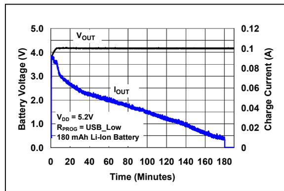
**FIGURE 2-28:** Complete Charge Cycle (180 mAh Li-Ion Battery).
