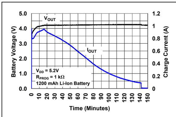
**FIGURE 2-26:** Complete Charge Cycle (1200 mAh Li-Ion Battery).
