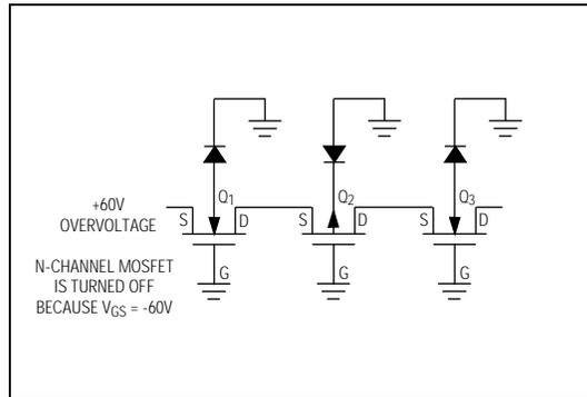
Figure 8. +60V Overvoltage with Multiplexer Power OFF
