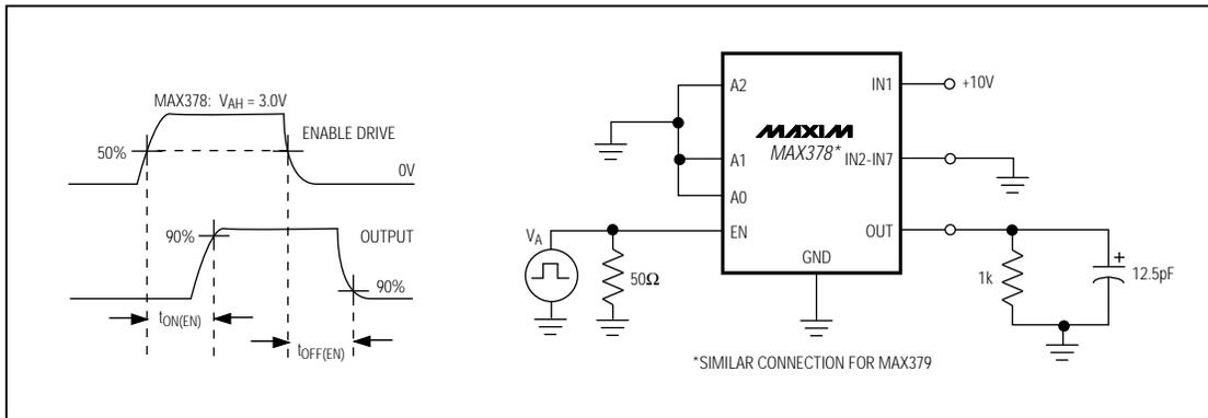
Figure 3. Enable Delay ( $t_{ON(EN)}$ ,  $t_{OFF(EN)}$ )
