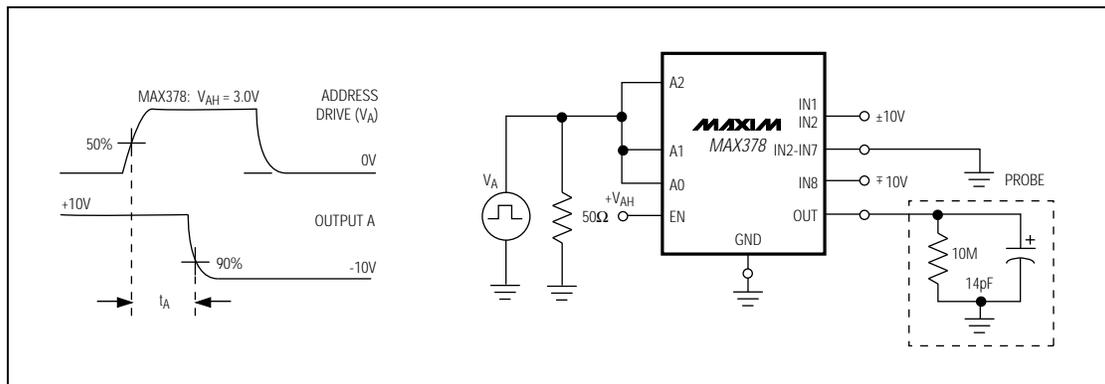
Figure 1. Access Time vs. Logic Level (High)
