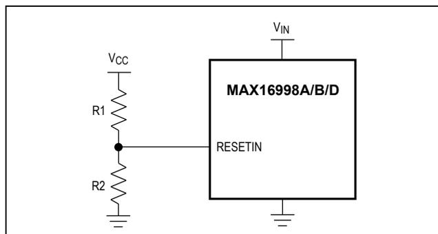
Figure 7. Setting RESETIN Voltage for the MAX16998A/B/D
