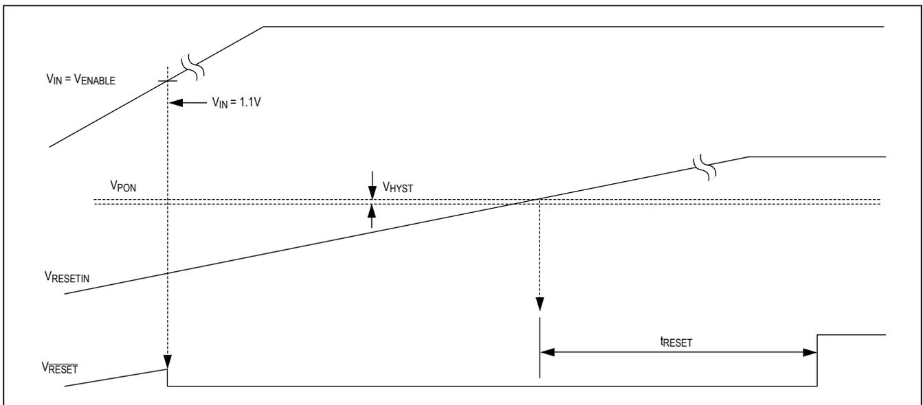
Figure 6. Detailed Power-Up Sequence for the MAX16998A/B/D
