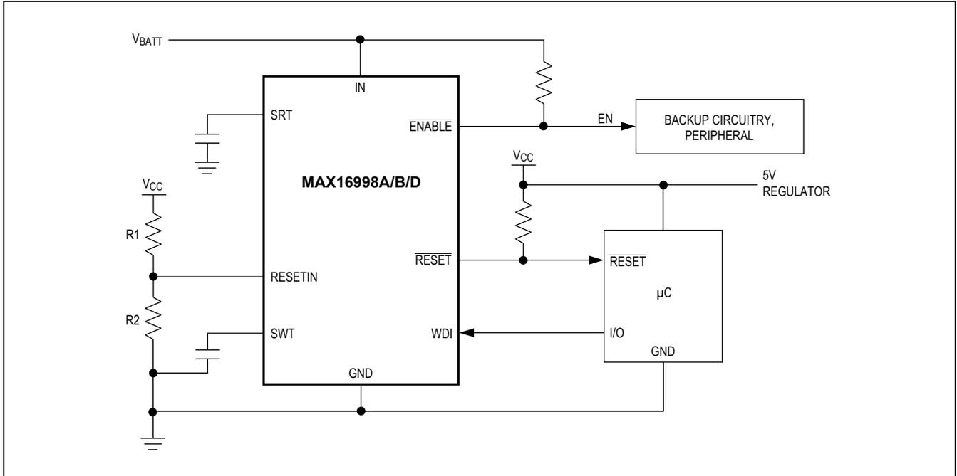
Figure 11. MAX16998A/B/D Switch Over to Backup Circuitry
