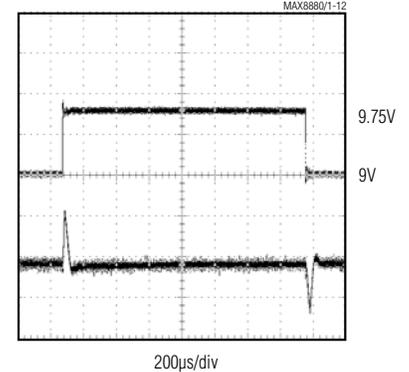
CH1 = V<sub>IN</sub>, 500mV/div, AC COUPLED
