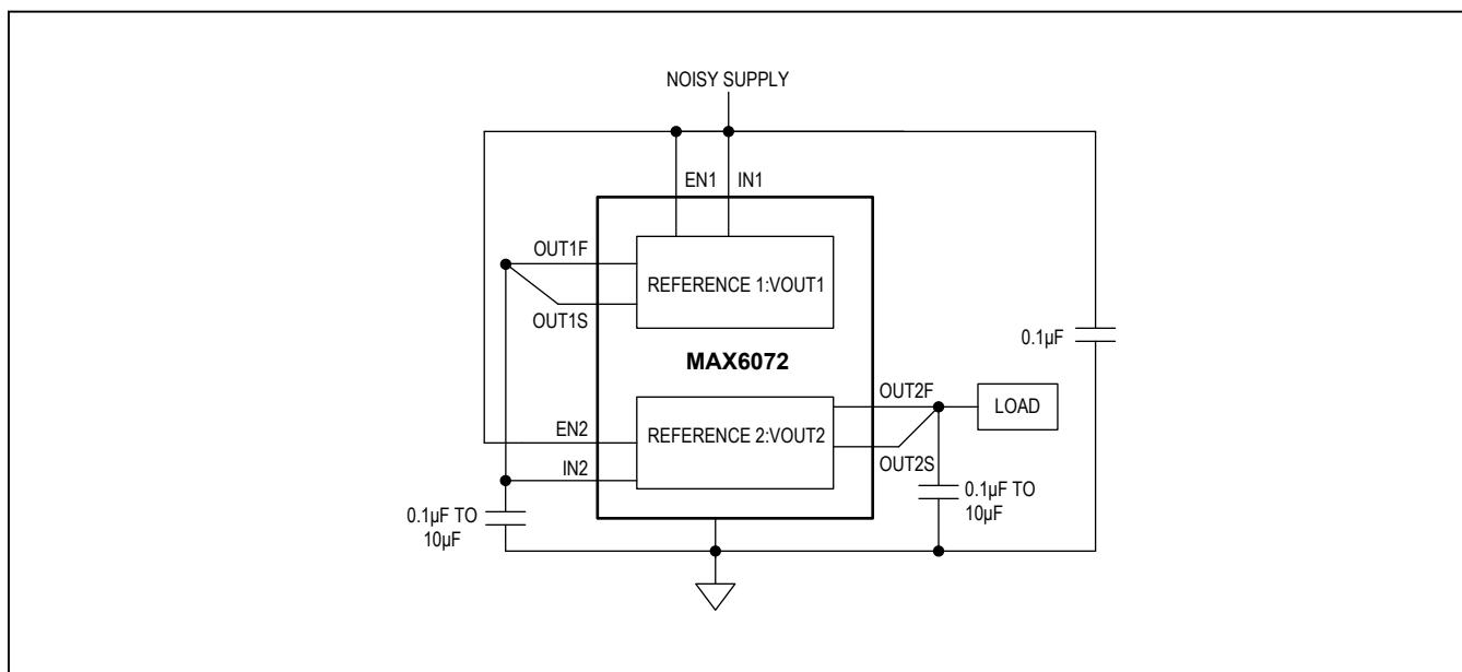
Figure 2. Increasing the Accuracy of Reference
