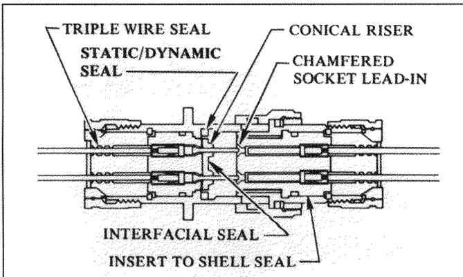
In addition to individual contact sealing, these connectors incorporate additional protective seals to assure sealing against environmental extremes: interfacial compression seal, peripheral static/dynamic
