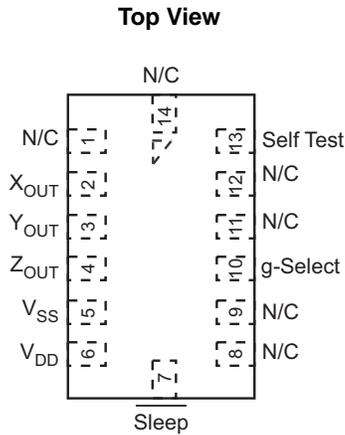
**Figure 4. Pinout Description**
