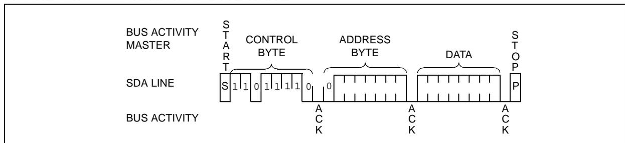
**FIGURE 6-2: SRAM/RTCC SEQUENTIAL WRITE**
