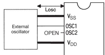
**Figure 2-3 Sample Oscillator Circuit 3 (External oscillator)**
