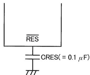
Figure 5 Reset Circuit
