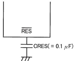
Figure 5 Reset Circuit
