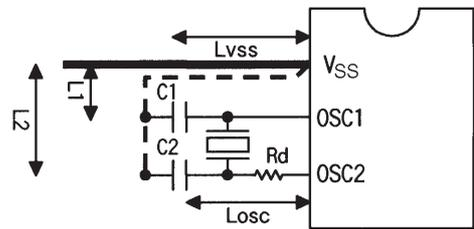
**Figure 2-1 Sample Oscillator Circuit 1 (Ceramic oscillator)**
