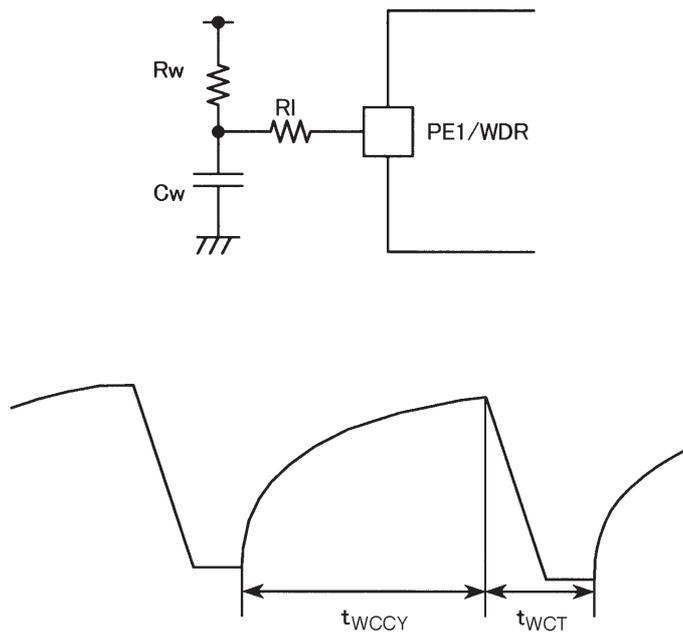
$t_{WCCY}$ : The charge time due to the time constant of the circuit consisting of the external components  $C_w$ ,  $R_w$ , and  $R_I$ .
