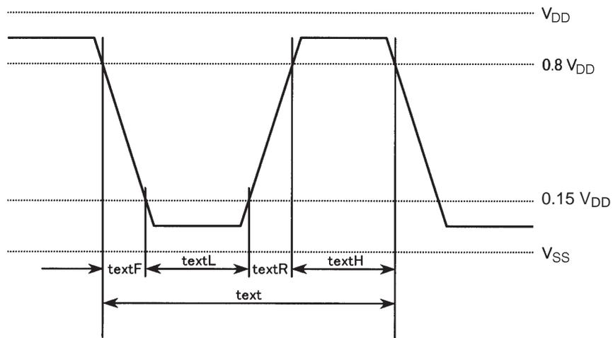
Figure 1 External Clock Input Waveform
