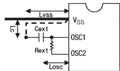
**Figure 2-2 Sample Oscillator Circuit 2 (2-pin RC oscillator)**
