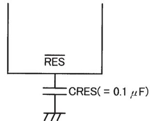
Figure 5 Reset Circuit
