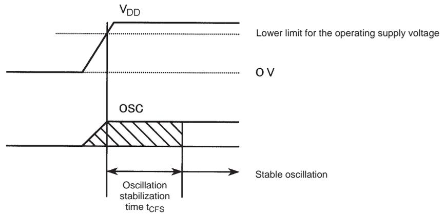
Figure 4 Oscillation Stabilization Time
