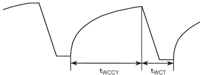
$t_{WCCY}$ : The charge time due to the time constant of the circuit consisting of the external components  $C_w$ ,  $R_w$ , and  $R_I$ .
