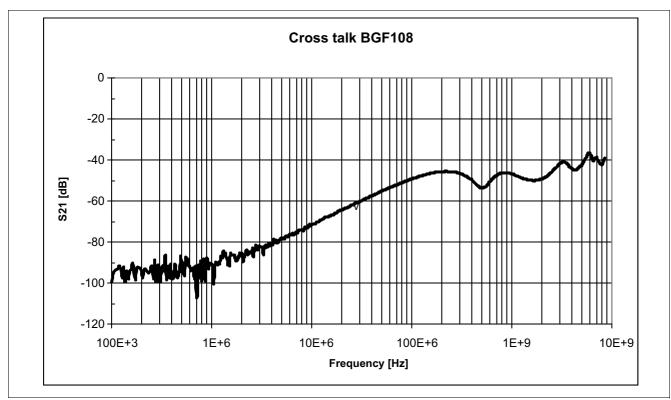
Figure 4 Typical cross talk between two channels ( $Z_{\rm S}$  =  $Z_{\rm L}$  = 50  $\Omega$ ,  $V_{\rm R}$  = 0 V)
