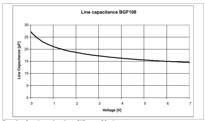
Figure 2 Capacitance of one line to GND versus DC voltage
