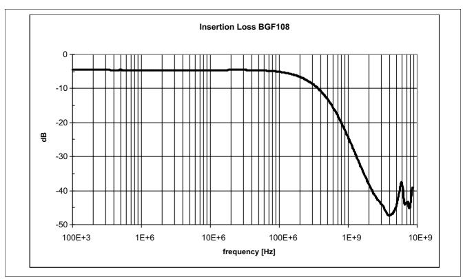
Figure 3 Typical filter characteristics of on channel ( $Z_{\rm S}$  =  $Z_{\rm L}$  = 50  $\Omega$ ,  $V_{\rm R}$  = 0 V)
