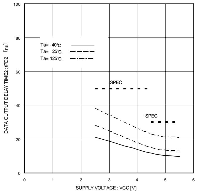
Figure 26. Data Output Delay Time tPD2 (CL=30pF)
