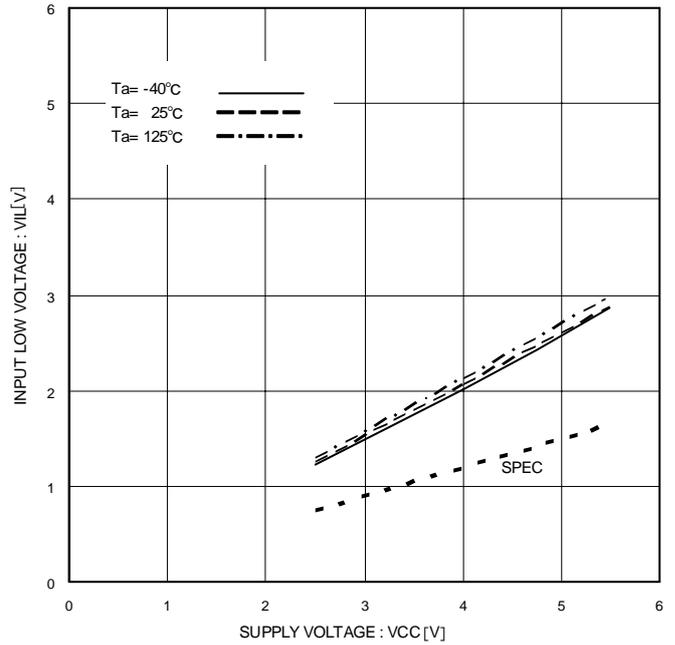
Figure 8. Input Low voltage  $V_{IL}$
