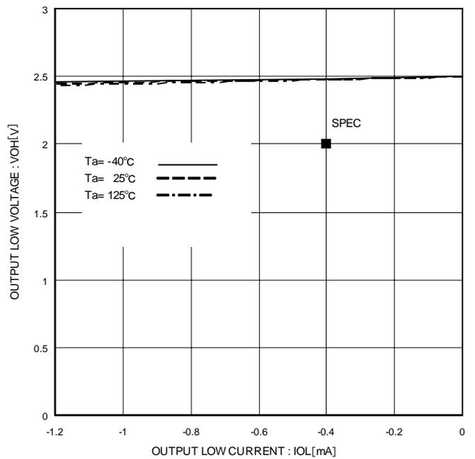
Figure 10. Output High Voltage  $V_{OH}$ ,  $I_{OH}$
