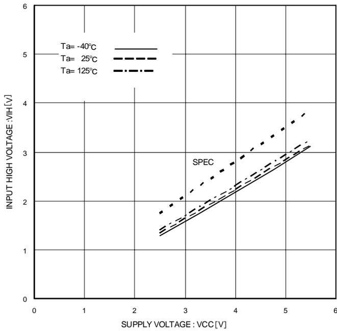
Figure 7. Input High Voltage  $V_{IH}$
