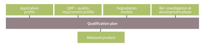
This thorough method allows prediction of useful life in customer application with target cumulative failure (FIT) rate.
