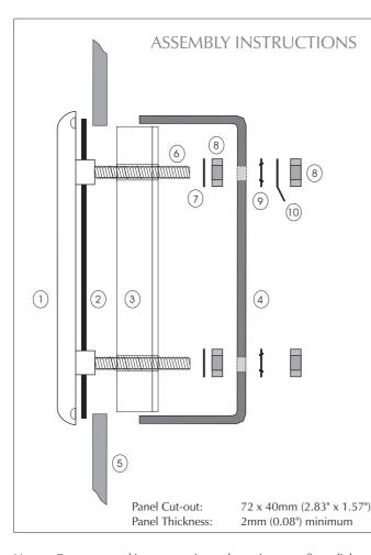
Bezel Qty. 1 ② O-ring Qty. 1 (3) Panel Instrument 4 Mounting Clamp Qty. 2 (5) Front Panel (6) Screw Stud Qty. 4 (7) Insulating Washer Qty. 4 Qty. 8 (8) Fixing Nut 9 Shakeproof Washer Qty. 4
