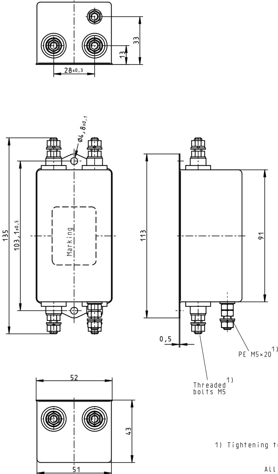
1) Tightening torque 2,6...3,0 Nm!
