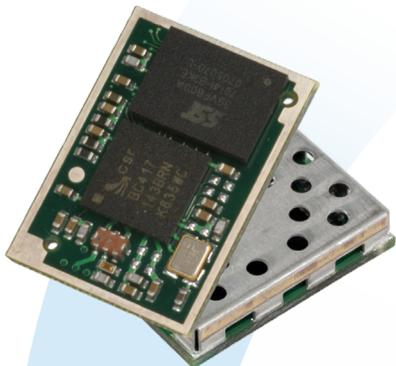
The BTM430 and BTM 431 Bluetooth® modules from Laird Technologies have been designed to meet the needs of developers who wish to add robust, short range Bluetooth data connectivity to their products. They are based on the market leading Cambridge Silicon Radio BC04 chipset, providing exceptionally low power consumption with outstanding range.
