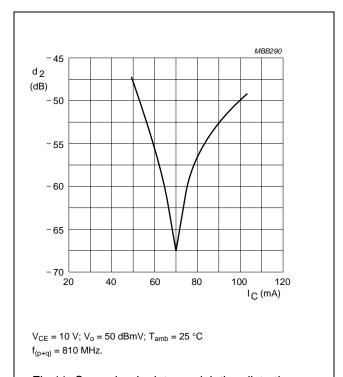
Fig.11 Second order intermodulation distortion as a function of collector current.
