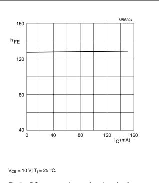
Fig.5 DC current gain as a function of collector current.
