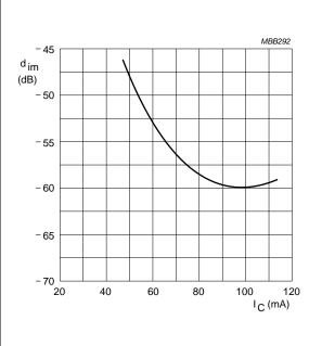
$V_{CE} = 10 \text{ V}; V_o = 900 \text{ mV}; T_{amb} = 25 \text{ °C}; f_{(p+q-r)} = 443.25 \text{ MHz}.$
