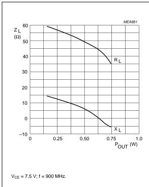
Fig.12 Load impedance as a function of output power.
