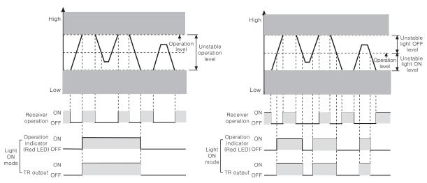
\*The waveform of 'Operation mode indicator' and 'TR output' is for Light ON mode, it is operated as reverse in Dark ON mode.
